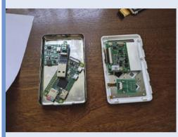
Carefully open up the MP3 player you're repurposing, remove its existing components, retaining anything you'll reuse, then check the replacement parts will fit within the chassis.
