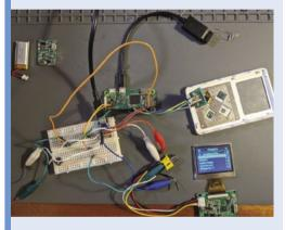
D2 Install the C-based haptic code on Raspberry Pi Zero. Connect Raspberry Pi, display, headers, and leads. Then power on and check the click wheel data is recognised and drives the haptic motor.
