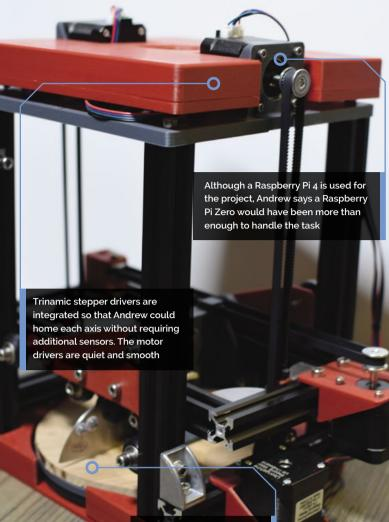
The device includes a plywood turntable which ensures the bread is in the correct position for cutting
