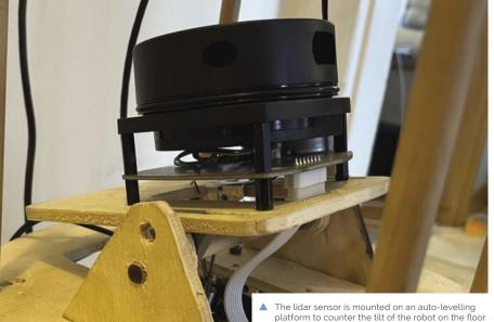
platform to counter the tilt of the robot on the floo – this will really come into play when Nick makes the robot self-balancing A Raspberry Pi in the head streams the camera feed to a master computer, and sends head movement commands to an Arduino
