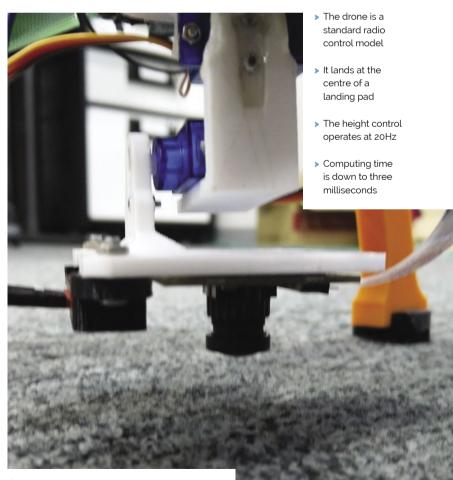
A gimbal was built by combining two servos with 3D-printed parts and this ensures the camera, which sits at the very bottom of the setup, is stabilised
