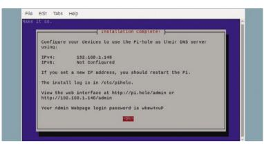
When you've finished setting up Pi-hole, make a note of the IPv4 address and password for later use existing list selected by pressing **TAB** to select OK and press **ENTER**. Ensure both IPv4 and IPv6 are selected on the 'Select Protocols' screen, and select OK.
