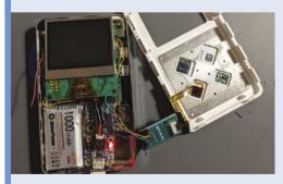
**D3** Tape off any conductive elements in the case to prevent short-circuiting. Test Raspotify and install on Raspberry Pi Zero before mounting it in your new music player and powering it up.
