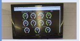
"All data is viewable in real time and historically, while all actuators are controllable via our Adafruit IO dashboard. Adjustment parameters like RGBW light spectrum, photoperiod, fan speed, pH and temperature set points, and liquid dosing volumes can be chosen here as well."
