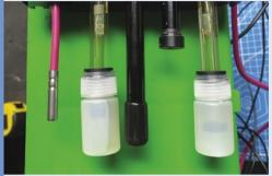
"The entire system has a network of sensors... which monitor atmospheric variables of air temperature, humidity, CO<sub>2</sub>, O<sub>2</sub>, and air pressure. Root zone variables include soil moisture by way of capacitive resistance sensors, reservoir levels by way of float switches, water/soil temperature, water/soil pH, nutrient levels by way of EC, dissolved oxygen, and water quality/root health by way of ORP (oxidation reduction potential)."
