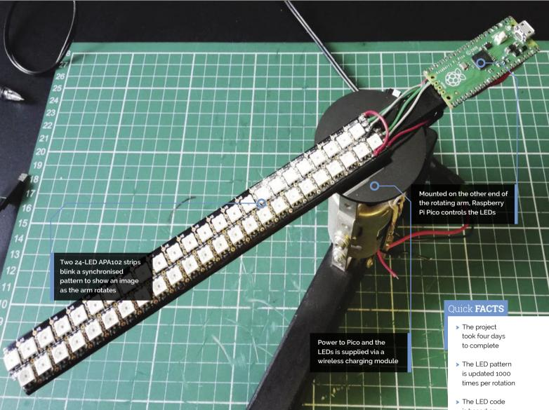
fast", they've managed to spin the arm at up to 960 rpm while displaying an image at 1000 frames per rotation.
