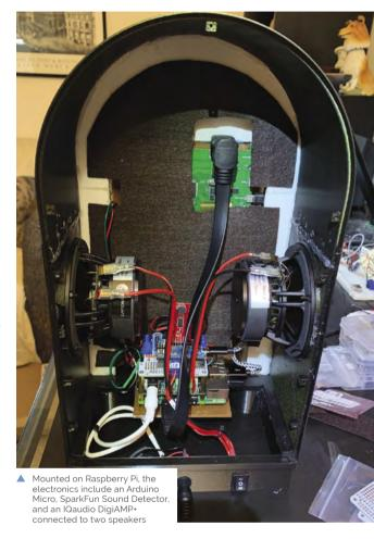
an Arduino Micro. The Arduino uses the Sound Detector output to power NeoPixel strings for sound-reactive lighting effects."
