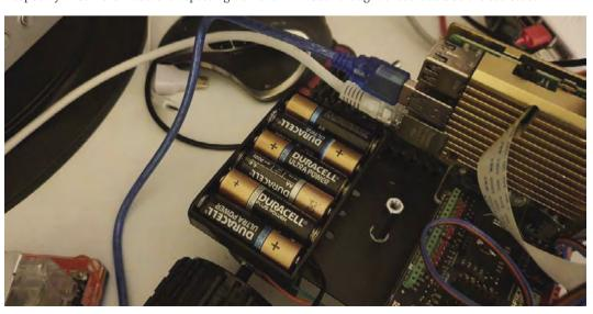
While the Arduino and motors are powered by six AA batteries, a highcapacity power bank is used for Raspberry Pi
