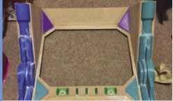
The cabinet was designed and laser-cut from MDF. There's some steel in the construction, as well as tempered glass over the screen. Mouldings are 3D-printed, with the help of a graphic artist who also helped rework graphics to fit the smaller size. Lastly, a riser is constructed to make sure it's tall enough to play.
