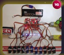
**Get your motor running** The current and voltage required for driving robot motors is not something that is going to keep your Raspberry Pi healthy for long. A robotics HAT is essential if you want your Raspberry Pi to control servos and motors. And to become truly portable, you'll need extra power too. For exceptional power and control, have a look at our RedBoard+ review in The MagPi issue 91 (magpi.cc/91).
