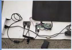
Lay out and connect Raspberry Pi, AV controller board, SD card, and display power cables. A four-gang power strip helps organise power supplies.
