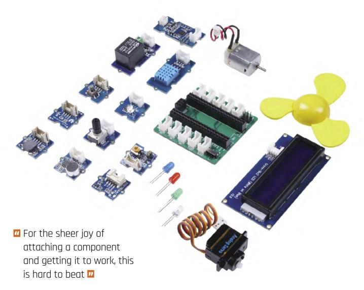
end, the kit comes with a wide range of parts to play with. There is an LED pack, RGB LED display, light sensor, sound sensor, rotary angle sensor, temperature and humidity sensor, passive buzzer, button, servo, mini fan (with DC motor), relay, and a 16×2 character LCD.
