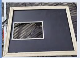
Setting up an LCD chalkboard is broadly similar to creating a magic mirror, for which detailed instructions are on GitHub (magpi.cc/magicmirrorgit). Apply chalkboard paint to one side of your plywood chalkboard, then cut out a hole the correct size and dimensions for your LCD. Measure and fit the frame.
