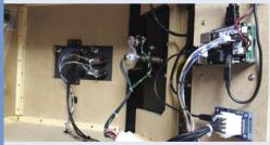
"The workings were simple when it came down to it: Raspberry Pi 3B+ with Pimoroni Picade X HAT. This gives us a power switch, audio amp, buttons, and a joystick if necessary. The replica yoke is interfaced with a USB adapter from the same company. It allows us to use the yoke with the original Atari connector. Software is RetroPie and I'm currently emulating on AdvMAME."
