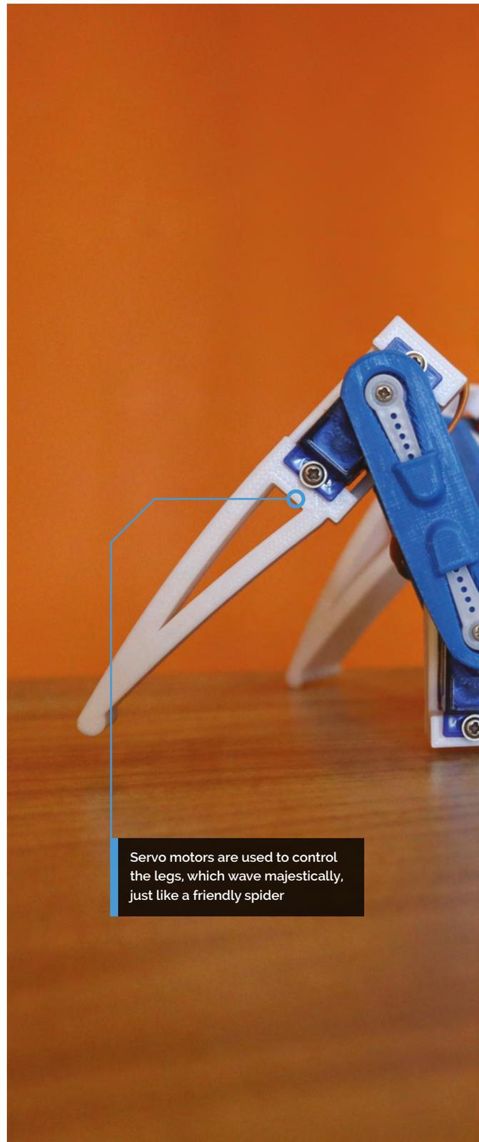
Servo motors are used to control the legs, which wave majestically, just like a friendly spider
