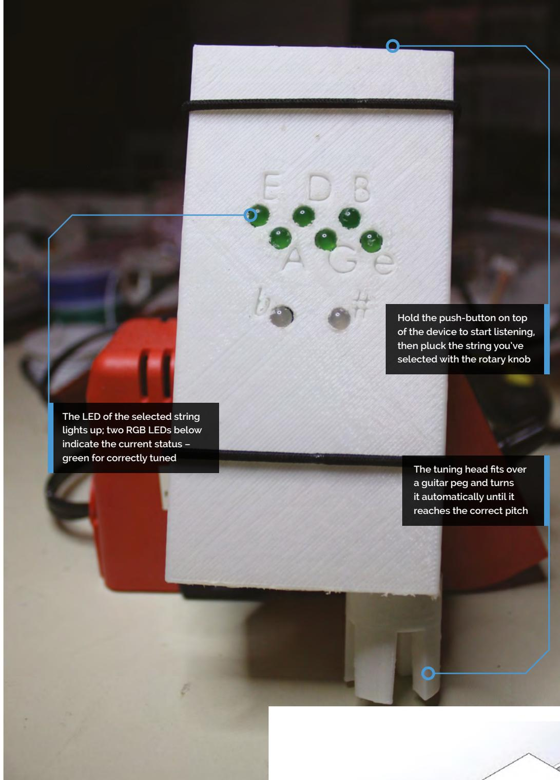
The LED of the selected string lights up; two RGB LEDs below indicate the current status – green for correctly tuned
