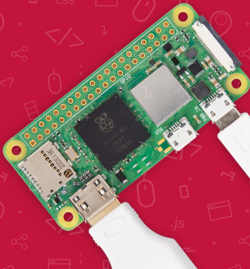
◀ You may need a micro USB to USB A adaptor and mini-HDMI to HDMI adaptor to connect devices such as a mouse, keyboard and display
