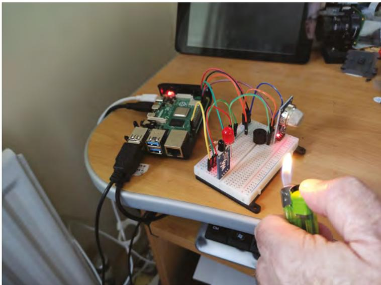
▲ Testing the flame sensor with a lighter. Be careful not to move it too near the sensor or other components!
