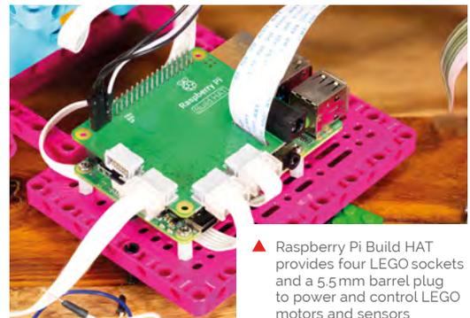
▲ Raspberry Pi Build HAT provides four LEGO sockets and a 5.5 mm barrel plug to power and control LEGO motors and sensors
