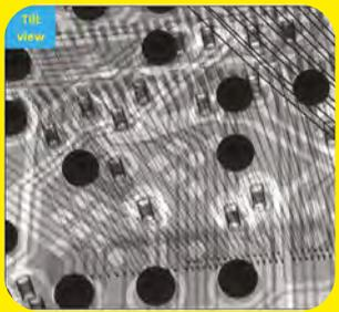
Here is a top-down X-ray of the System-in-Package that reveals an Easter egg! Spot the Raspberry Pi logo shape in the ball map. This is possible because, while the connections on the outside are signals, the ones in the middle are ground/power and can be arranged into any pattern.
