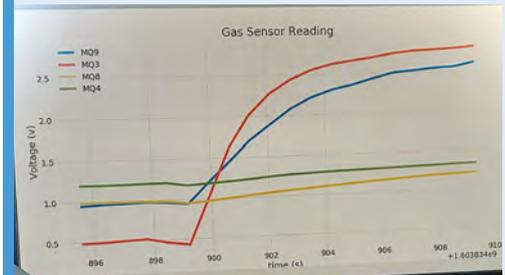
**01** The sensors are calibrated when it turns on – this is done by having the Python script run on start up, and holding the sensors away from anything you'd like to whiff. Once the sensors are calibrated to neutral, a sensor reading will be displayed.
