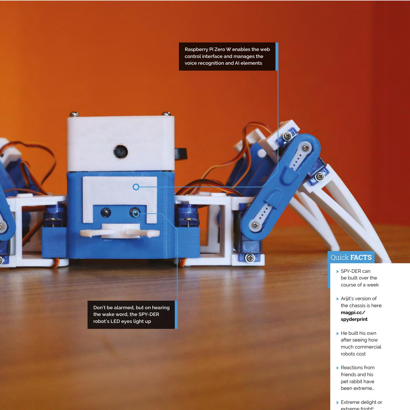
Raspberry Pi Zero W enables the web control interface and manages the voice recognition and AI elements
