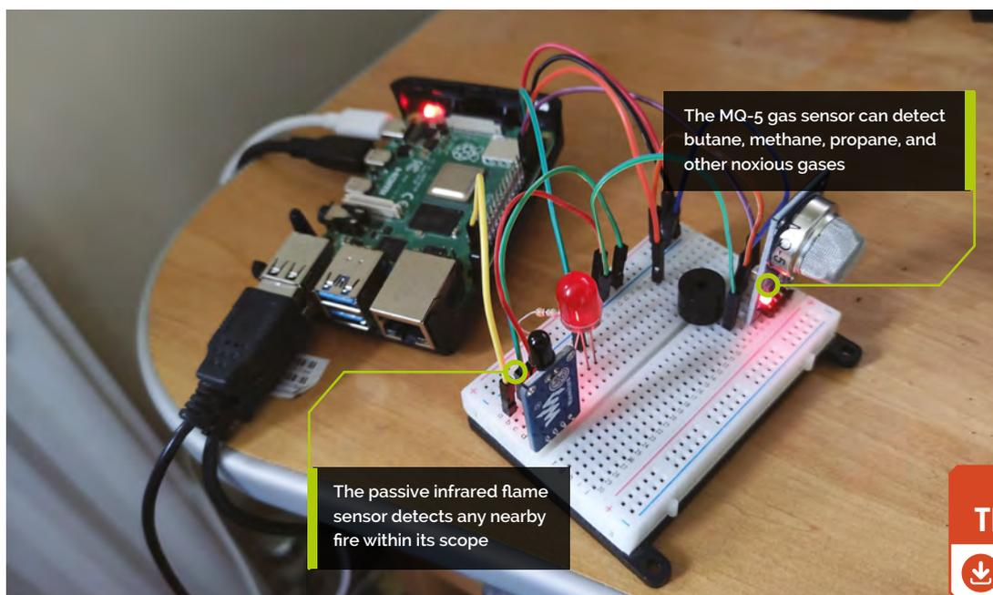
our code, we import the `Button` method from it. We'll use this to sense when the digital output from the sensor is high, in effect the equivalent of a push-button being pressed. As it's connected to GPIO 21, we assign the `flame` object to this with `flame = Button(21)`.
