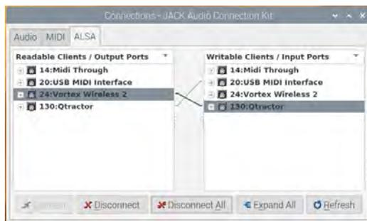
**▲** Above Here, we're using Jack's Connect interface to connect Qtractor to our MIDI interface, and our Vortex Wireless MIDI keytar to Qtractor. Think of the lines as patch cables
