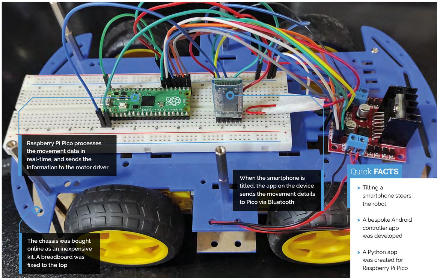
Raspberry Pi Pico processes the movement data in real-time, and sends the information to the motor driver
