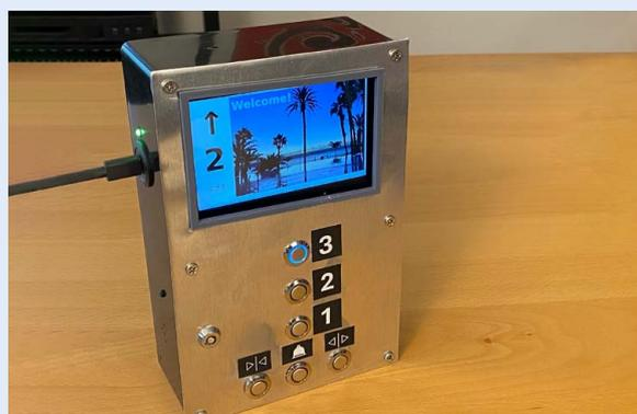
2. The display is driven by a web browser container in kiosk mode. A tiny web server runs in a separate container to serve the page. The main Python code establishes a web socket with the server to update the static web page. It uses the Pygame library to play audio.
