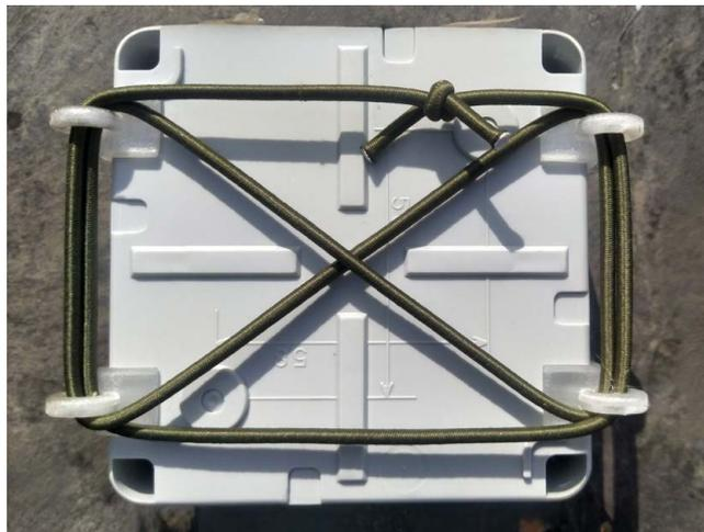
◀ **Figure 7:** Some PETG 3D-printed eye mounts were superglued onto the outside of the enclosure. Through these we added some stretchy shock cord, allowing the node to quickly be attached to poles and other objects
