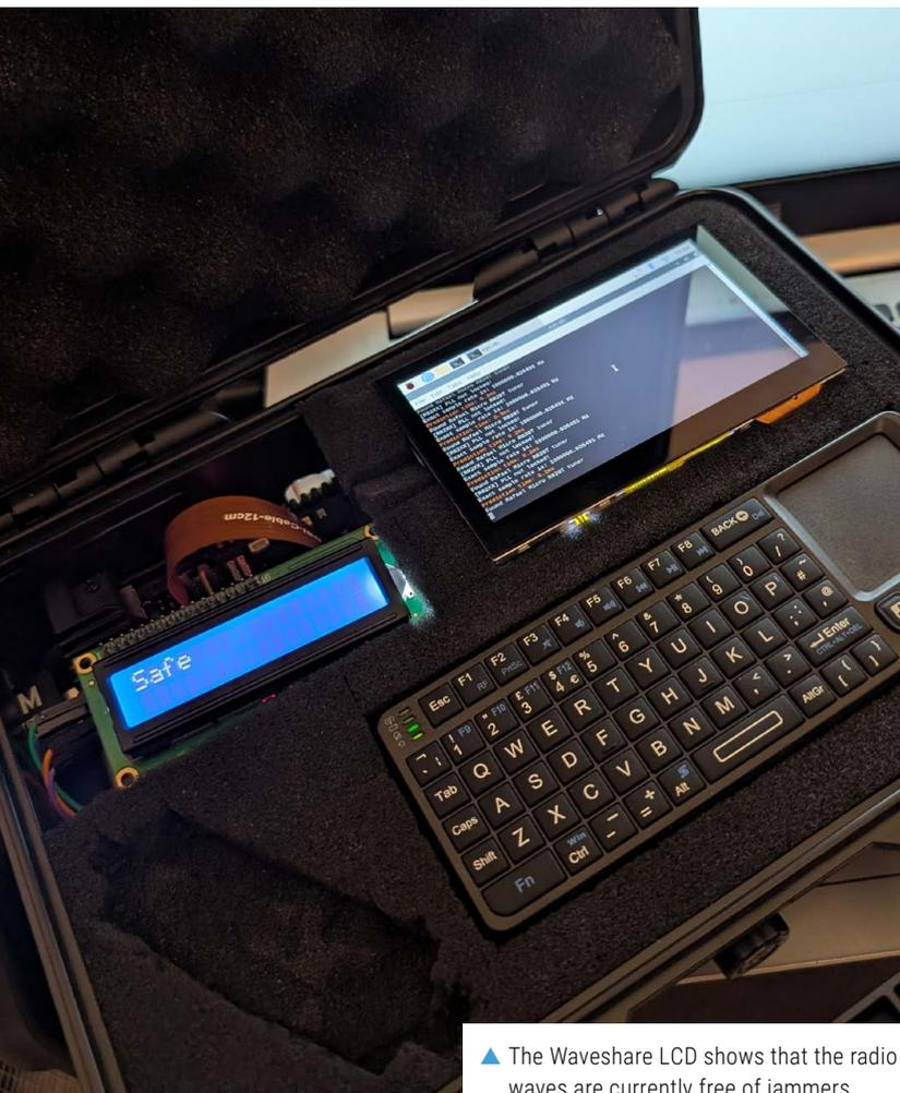
▲ The Waveshare LCD shows that the radio waves are currently free of jammers
