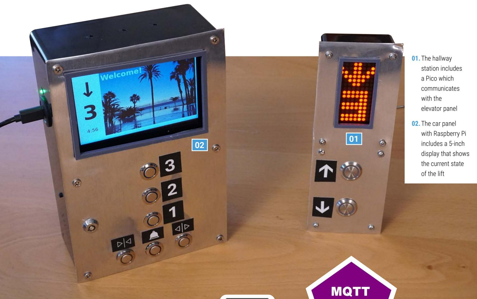
**01.** The hallway station includes a Pico which communicates with the elevator panel
