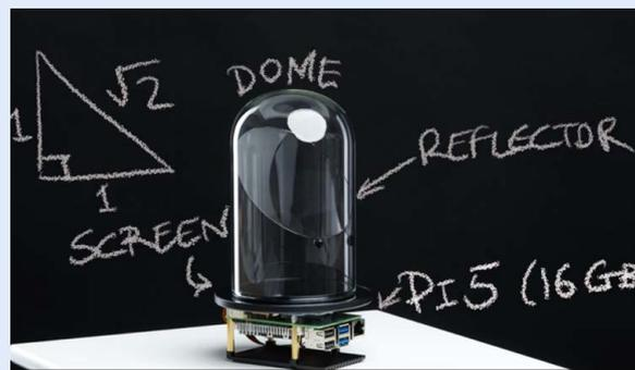
2. Set up the source image and mirrors, using the handy reflector shape calculator on Veeb's website: [rpimag.co/pepperpi](http://rpimag.co/pepperpi). Veeb used MPV ([mpv.io](http://mpv.io)) and some tweaks to Raspberry Pi OS to include video effects.
