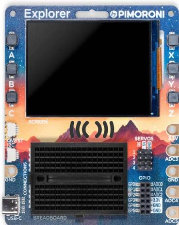
**N**ot to be confused with the classic Explorer HAT Pro (still a great option for Raspberry Pi computers), this standalone Explorer is based around the RP2350 microcontroller chip – as used in Raspberry Pi Pico 2 / 2W, so it's programmable with MicroPython and C/C++.
