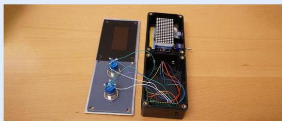
3. The other panels have Picos inside and run on CircuitPython, which also has a compatible MQTT library. The hydraulics use a Pico W to power relays that allow sufficient water in and out of the system to move the elevator car up and down.
