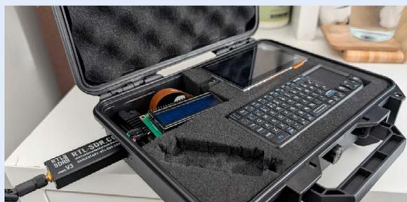
2. Cut a hole to accommodate the SDR-dongle so it can be used from inside the case. Install drivers for the RF-SDR dongle from the libstlsdr library. Attach the I2C LCD to Raspberry Pi's GPIO pins.
