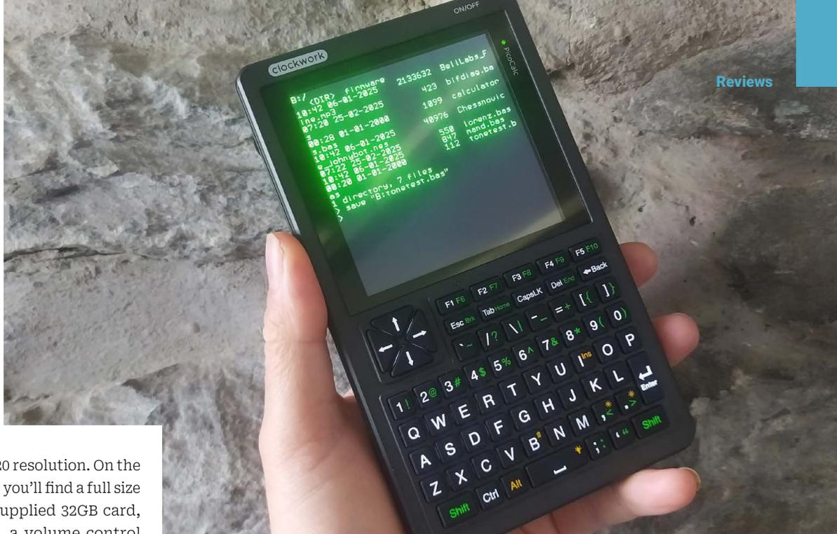
brightness and 320×320 resolution. On the assembled main board you'll find a full size SD card slot with a supplied 32GB card, a headphone socket, a volume control and a horizontal header that is used to access the GPIO from both the core board (Raspberry Pi Pico as standard) or the STM32. You'll also spot the battery socket which is designed for up to two 18650 cells, although it can be powered by a single cell.
