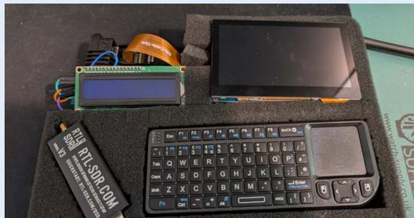
1. You will need an RF-SDR dongle, Raspberry Pi display, I2C LCD, Raspberry Pi, mini keyboard, and a power supply. Carve spaces for each in the protective foam of a flight case and cut a hole in its side for a power cable.
