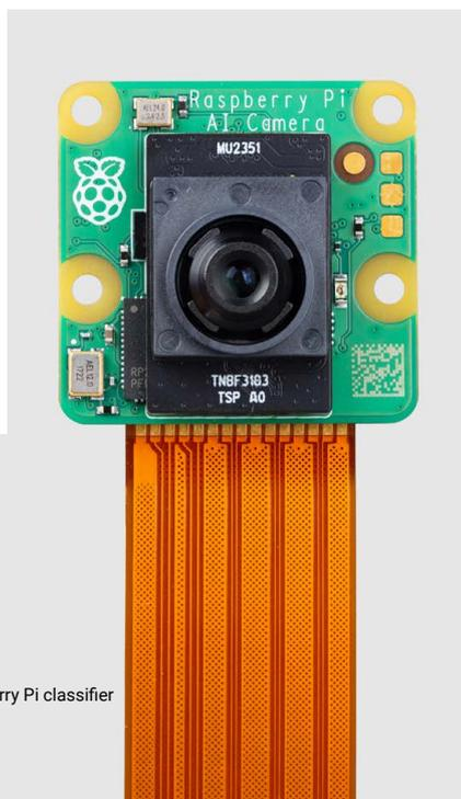
**I**n this tutorial, we will use Raspberry Pi AI Camera with a pre-trained model to detect different Raspberry Pi models. Point Raspberry Pi AI Camera at a Raspberry Pi 4 and it will display 'Raspberry Pi 4' on the screen, or 'Raspberry Pi Zero' and so on.
