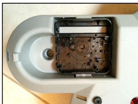
Figure 2a - Clock mechanism removed with lever gear visible
