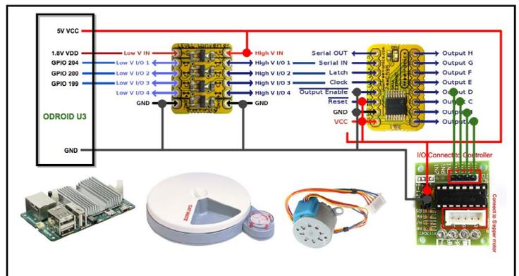
Figure 4 - ODROID Internet-controlled cat feeder schematics
