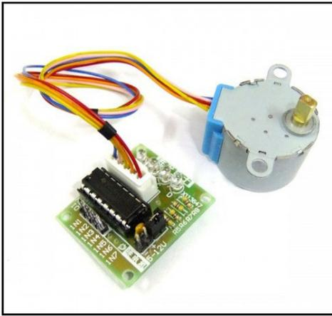
Figure 3a - 28BYJ-48 5V stepper motor with ULN2003 Driver Board
