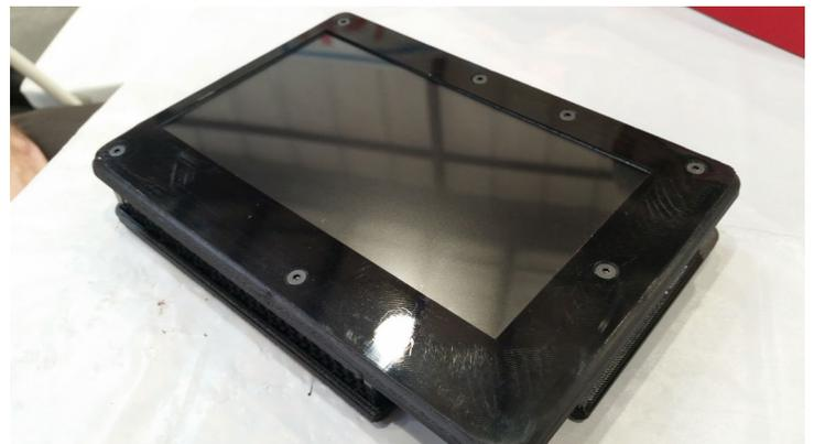
**Figure 12 - The completed tablet in all of its glory! You can optionally glue the included screw covers over top of the screws to give it a more finished look**
