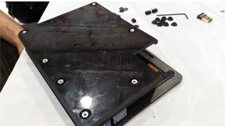
**Figure 8 - Place the back cover over top of the screws, and loosely place the nuts over the back cover with a single turn**
