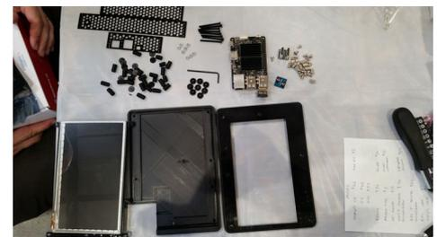
Figure 1 - Parts of the VU7 Tablet Kit
