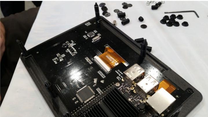
**Figure 7 - Place a pair of spacers over top of the 4 tablet cover screws, which may need to be trimmed slightly with a utility knife in order to ensure the best fit**
