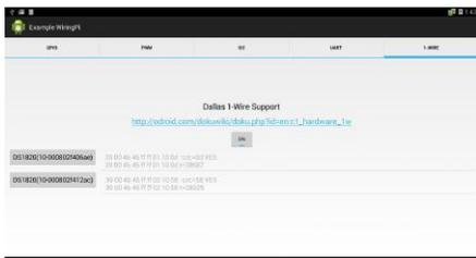
Figure 16 - Demo software to access 1-wire protocol interfaced DS18S20 temperature sensor
