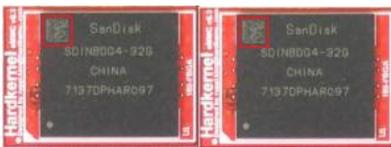
Figure 2 – eMMC version 5.0 (left) has the QR code on the right side, and eMMC version 5.1 (right) has the QR code on the left side)
