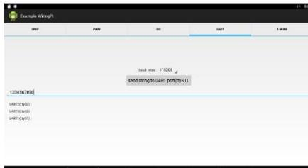
Figure 3 - Test the daisy-chained UART by typing a string
