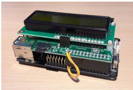
Figure 3 - The PiFace mounted on top of the ODROID-C2
