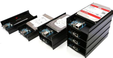
Figure 6 – The ODROID-HC2 is stackable
