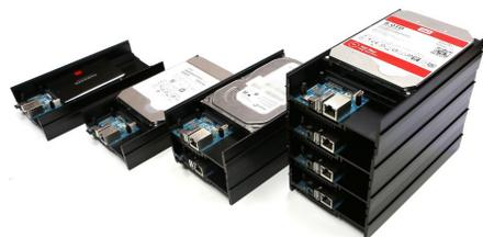
Figure 6 – The ODROID-HC2 is stackable
