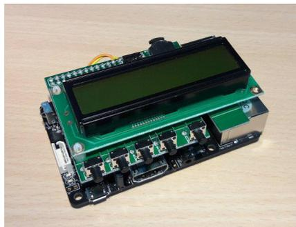
Figure 2 - Another view of the assembled PiFace and ODROID-C2
