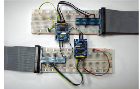
Figure 7 – connecting the CANL and CANH pins of two ODROID-C1 boards
