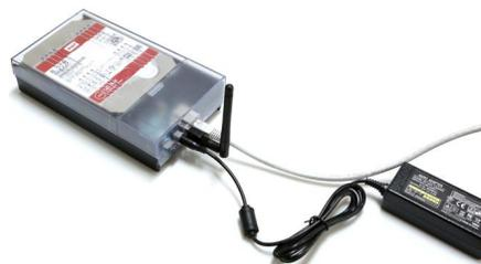
Figure 2 - A typical ODROID-HC2 setup with an 8GB microSD card, 3.5-inch hard drive, 12V/2A power supply, Ethernet cable, and ODROID-HC2 case
