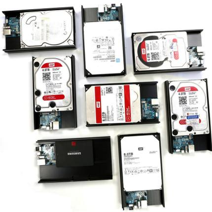
Figure 7 – The ODROID-HC2 was tested with various 3.5inch drives as well as 2.5inch storages
