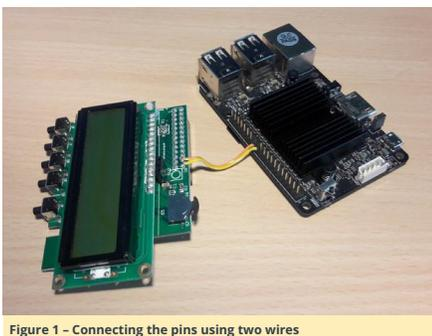
Figure 1 - Connecting the pins using two wires
