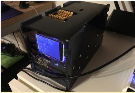
**Figure 3 – Cristian 3D-printed a custom top for his ODROID-XU4 that has space for the heat sink**
