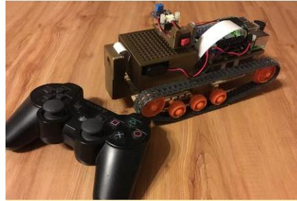
**Figure 4 – Cristian created a custom roving robot, controllable with a PS3 controller or web interface**
