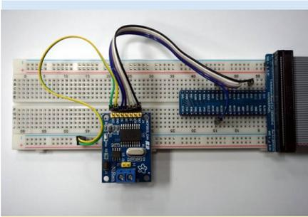
Figure 6 – Connect the CAN module and ODROID-C1 using tinkering kit
