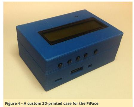
Figure 4 - A custom 3D-printed case for the PiFace
