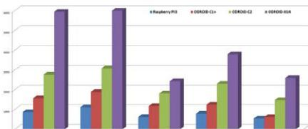
Figure 3 – CPU/RAM performance of the ODROID-XU4 vs the ODROID-C1+, ODROID-C2, and Raspberry Pi 3 using the Unixbench: Dhrystone-2, Unixbench: Double-Precision Whetstone (x3), Nbench 2.2.3: Integer (x40), Nbench 2.2.3: Floating-Point (x100), and mbw 100: Memory Bandwidth (MiB/s) benchmarks
