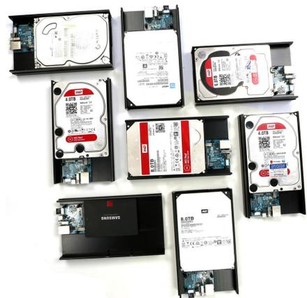
Figure 7 – The ODROID-HC2 was tested with various 3.5inch drives as well as 2.5inch storages
