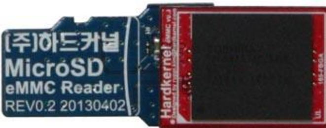
Figure 3 - eMMC module with reader
