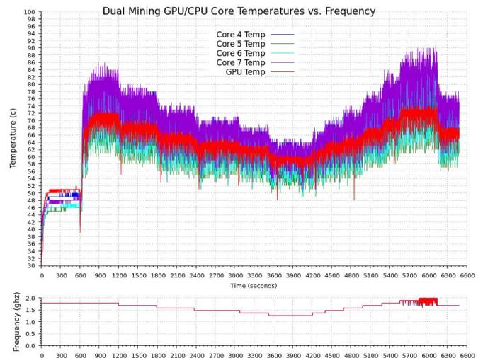
**Figure 3 – Dual Mining GPU/CPU Core Temperatures vs. Frequency**
