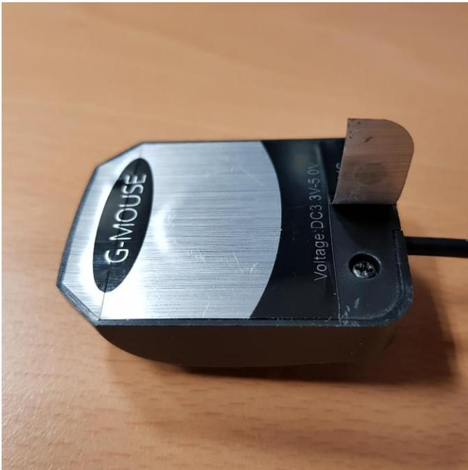
Figure 2 - Peel off sticker to access screws
