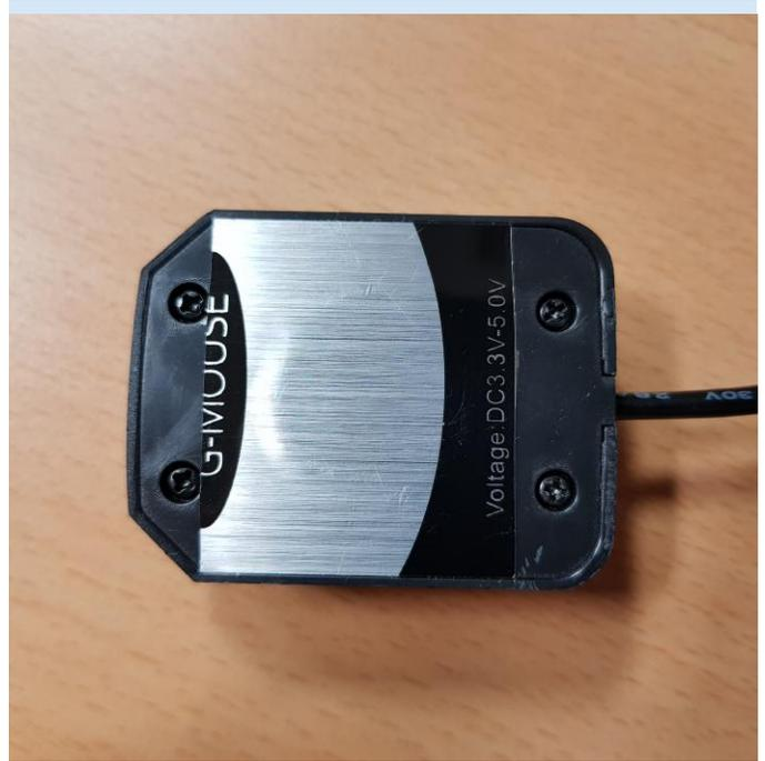
Figure 3 - Peel off sticker to access screws
