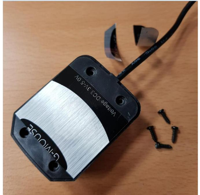
Figure 4 - All screws removed
