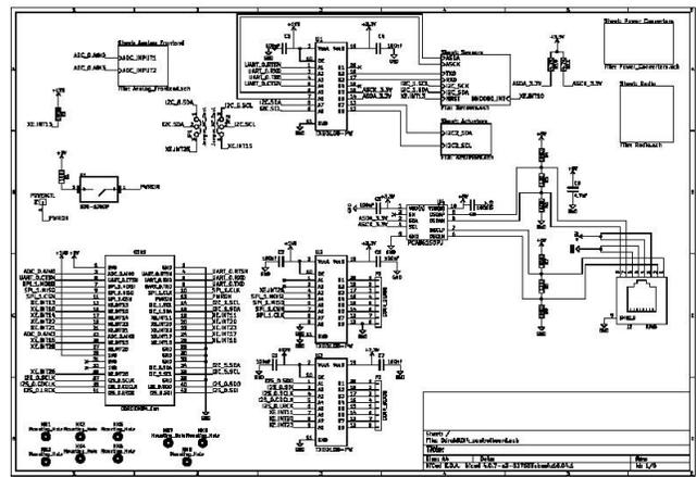
Figure 2 - Sensor board top level schematic, with ODR01D-XU4 connections, logic conversion, on-off button, and I2C to differential I2C conversion and RJ45 connector
