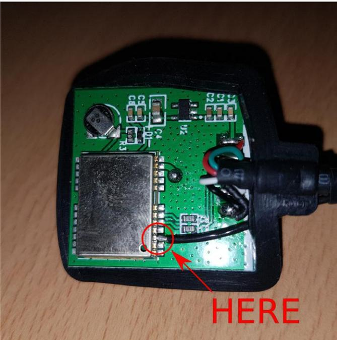
Figure 6 - PPS pin on main PCB
