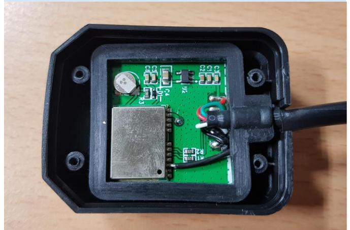
Figure 8 - Place PCB back into case
