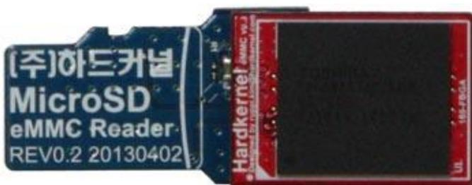
Figure 3 - eMMC module with reader
