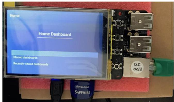
**Figure 3 – Grafana Dashboard in QtWebEngine Running on ODROID-C2 built using Yocto Project**
