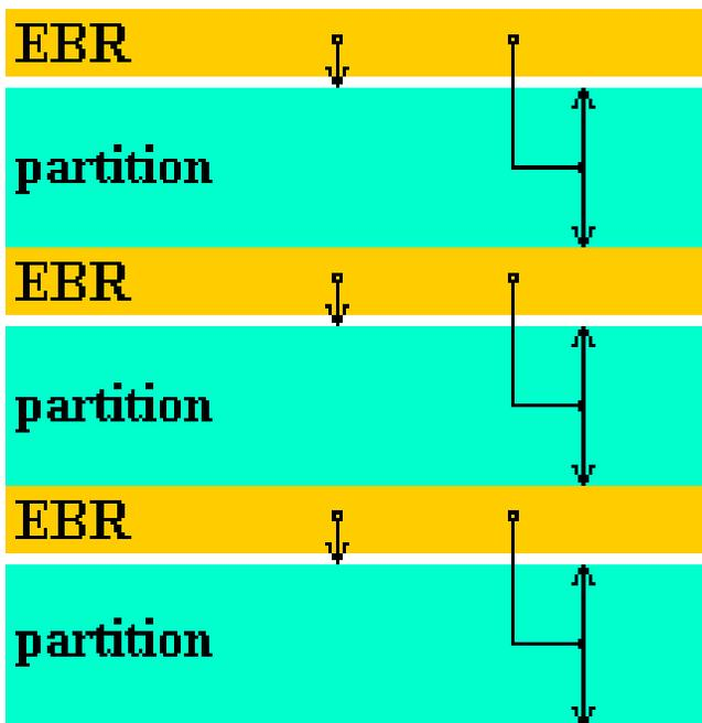
Figure 2 – EBR position on disk
