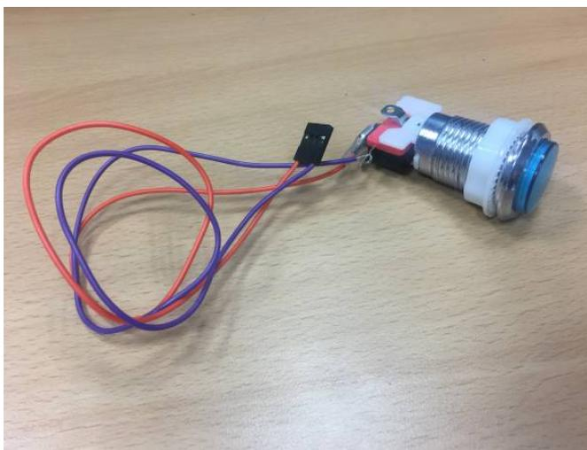
**Figure 4 - We prepared two buttons for use as a shut-down switch. For this project, we used the bigger button**
