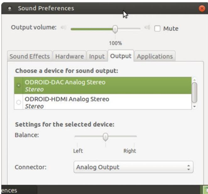
Figure 13 – Select Output: ODROID-DAC Analog Stereo
