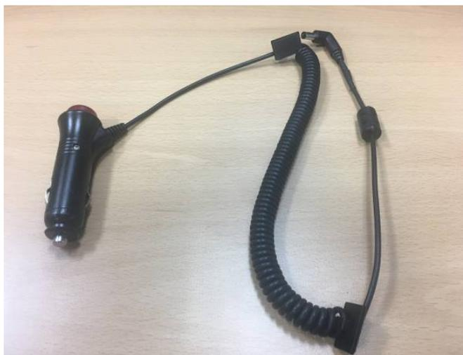
**Figure 5 - We used a cigarette lighter power adapter as power supply**
