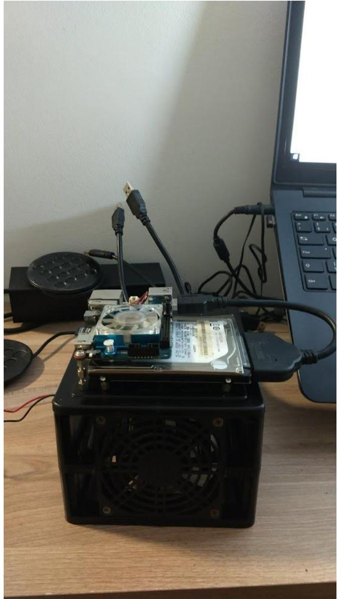
Figure 19 - Let's not forget the star of the show. Enter the ODROID-XU4 (and a fan too)
