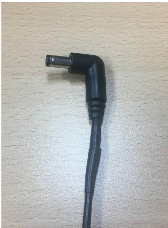
**Figure 6 - To connect the power adapter to SmartPower2, we changed the connector to a 5.5mm L type cable**
