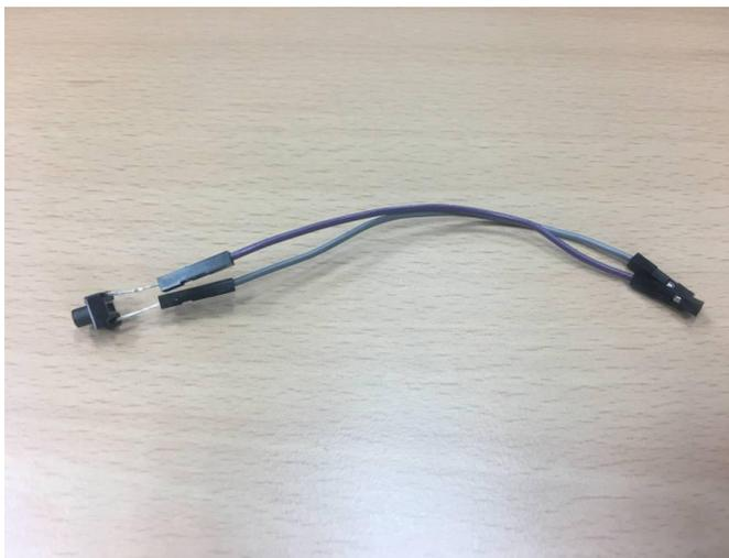
**Figure 3 - We prepared two buttons for use as a shut-down switch. For this project, we used the bigger button**
