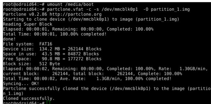
Figure 4 – Partclone backup with prior unmounting of /media/boot
