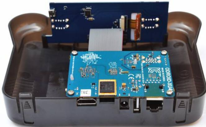
Figure 3 - Assemble the XU4 + LCD board in the top case (A) and fasten the screws (H)
