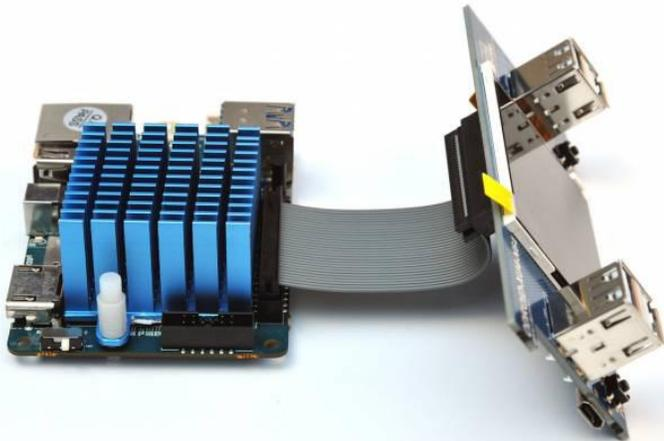
Figure 2 - Use a 30-pin flat cable (E) to connect the XU4 and the LCD board (C). Then remove the LCD surface protect film. The ODROID-XU4 is sold separately
