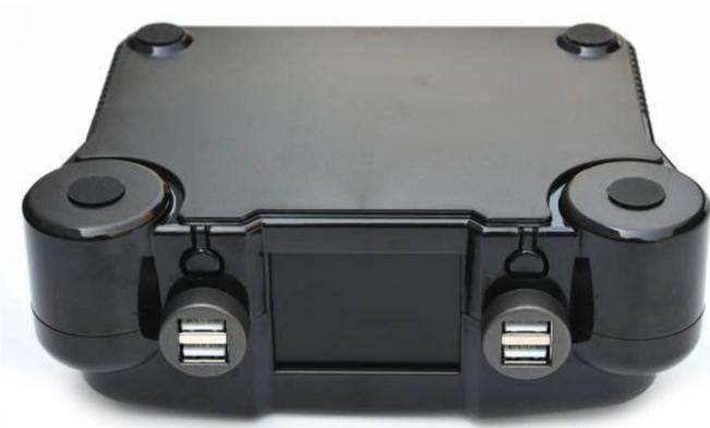
**Figure 8 - Assemble the bottom case (B) and fit the USB covers (F). Then attach the rubber feet (G) to the bottom case**
