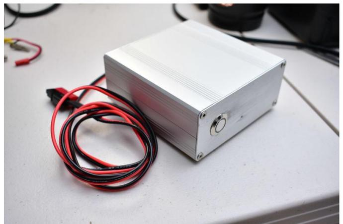
Figure 17 - Here is the box fully assembled. The holes for the USB, network connector and the power button were cut by hand and there was some scuffing. This can be avoided using painters tape or with better tools like a CNC or a bench drill
