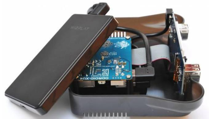
Figure 6 - Connect the XU4 board and the LCD board with the USB2.0 cable (D)
