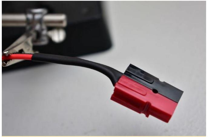
Figure 9 - I added some heat-shrink tubing to work as cable strain support
