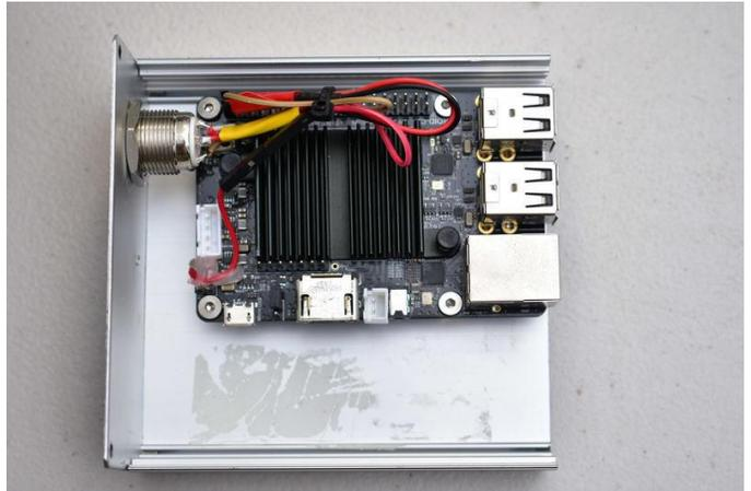
Figure 10 - The ODROID mounted using brass standoffs. The residue is from double-sided tape from a previous attempt
