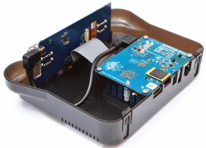
Figure 5 - Connect the XU4 board and the LCD board with the USB2.0 cable (D)
