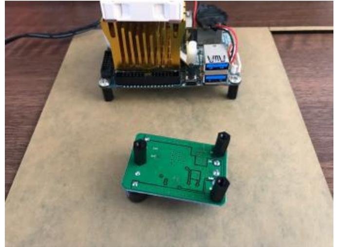
**Figure 4 - The standoffs for the XU4 and the DC-DC converter**
