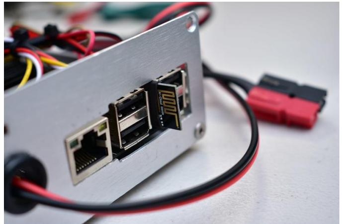
Figure 16 - The ESP8266 (ESP-01) programmed to work as a WiFi to serial console bridge. This will allow access to the console of the ODR0ID even if communications fail. This is perfect for debugging and management
