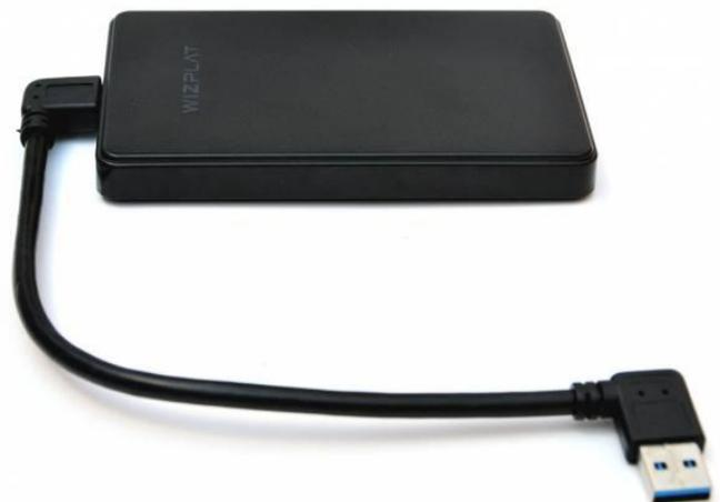
Figure 7 - You can connect a 2.5" HDD box using USB3.0 cable(I) included in the package and secure the HDD enclosure to the bottom case with velcro tape. The package does not include an HDD. If your USB HDD storage consumes more than 500mA, you might need to use a 5V/6A PSU instead of 5V/4A PSU
