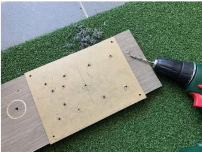
**Figure 7 - Drilling the acrylic sheet**
