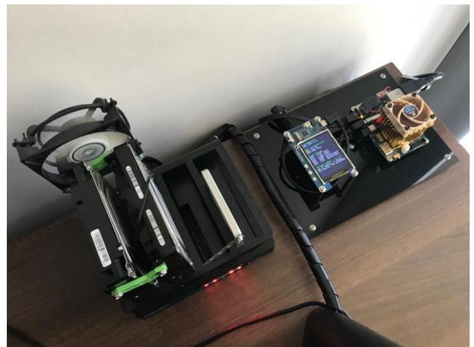
**Figure 10 - The final view of the server with cable management and acrylic sheets**
