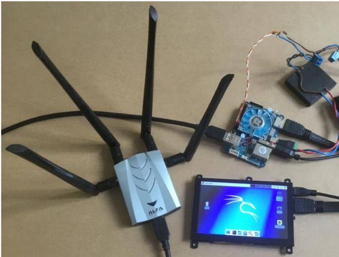
**Figure 1 - Kali Linux 2018.2 on ODROID-XU4 with Alfa WiFi adapter connected**
