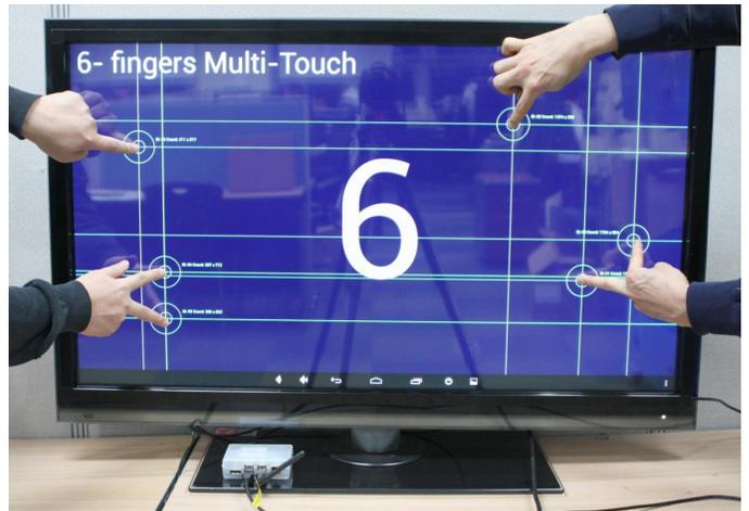
Figure 13 - Testing the touch screen
