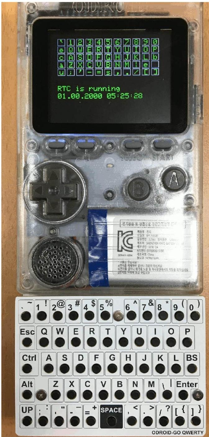
Figure 1 - Keyboard for the ODROID-GO
