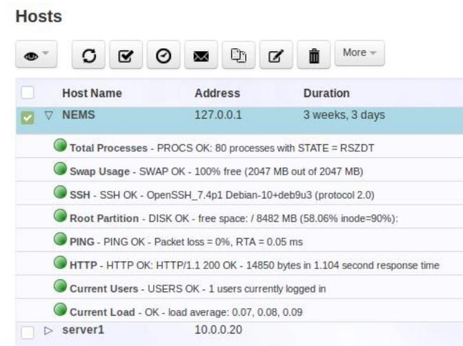
**Figure 7 - Expanded view of Host reveals configured service checks**
