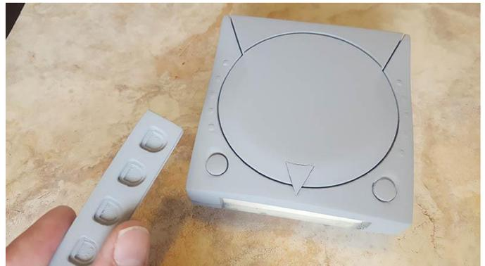
**Figure 14 - We had to drill a small hole through power button stem so we could secure with a paperclip**
