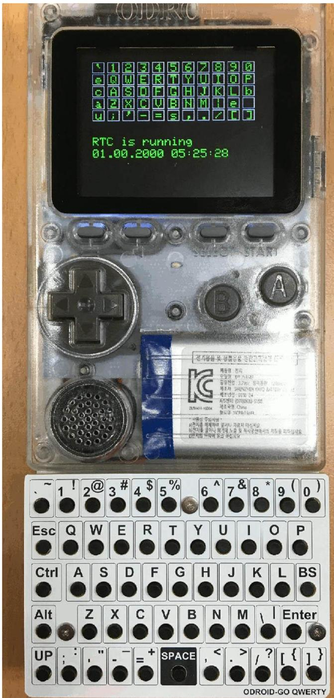
Figure 1 - Keyboard for the ODROID-GO
