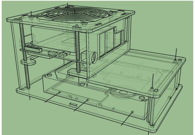
Figure 24 - Design prototype for ODROID-H2 case
