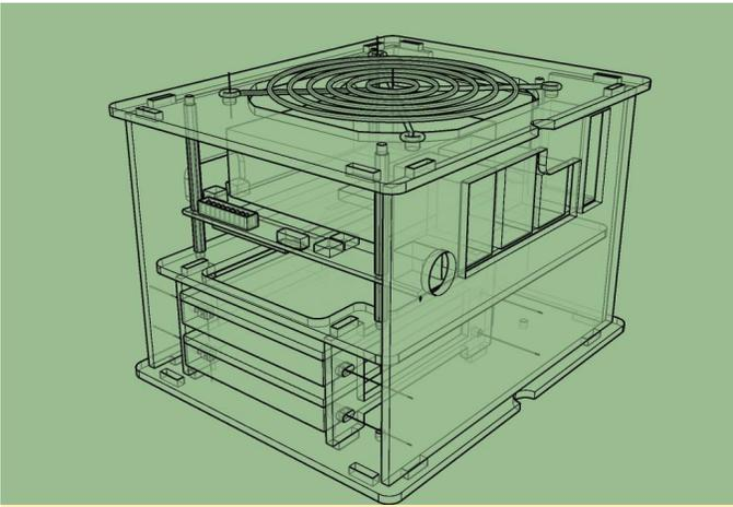
Figure 20 - Design prototype for ODROID-H2 case
