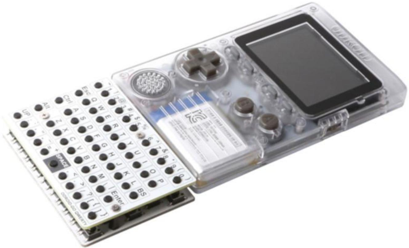
With Hardkernel's new bluetooth keyboard, you can turn your ODROID-GO to a portable handheld computer. ODROID-GO can emulate some classic computer systems such as Commodore 64, ZX Spectrum, and MSX. We believe a physical keyboard provides a better emulation experience for these systems.
