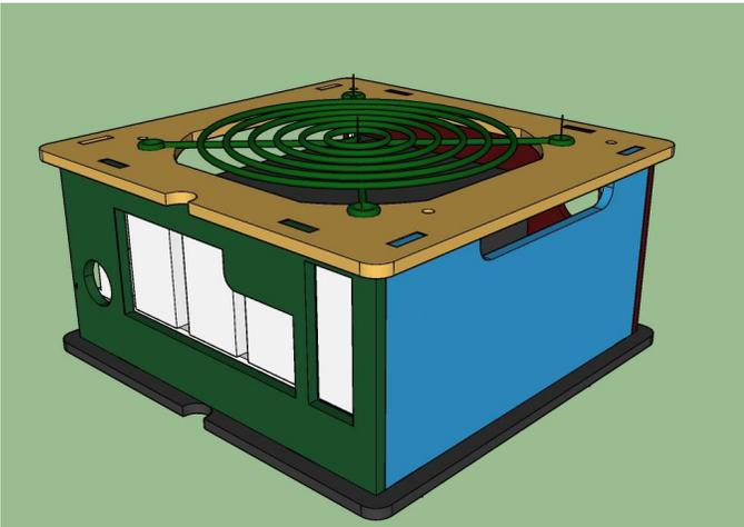
Figure 16 - Design prototype for ODRROID-H2 case
