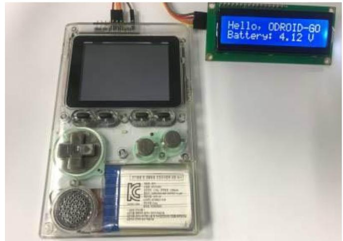
**Figure 03 - LCD with cable**
