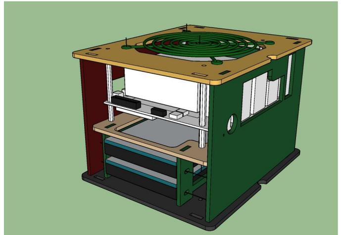
Figure 19 - Design prototype for ODRROID-H2 case
