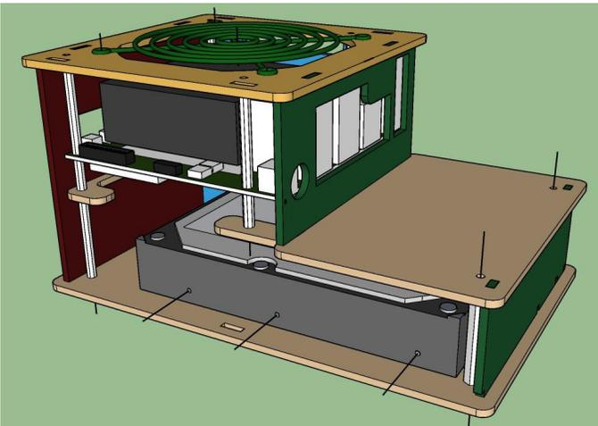
Figure 22 - Design prototype for ODROID-H2 case
