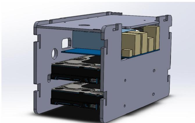
Figure 13 - Design prototype for ODROID-H2 case
