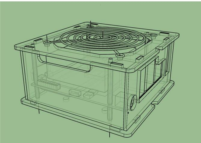
Figure 17 - Design prototype for ODRROID-H2 case
