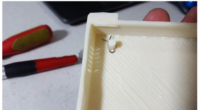
**Figure 12 - We had to drill a small hole through power button stem so we could secure with a paperclip**
