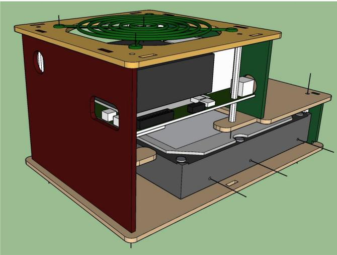
Figure 21 - Design prototype for ODROID-H2 case
