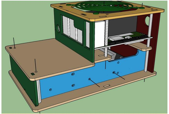
Figure 23 - Design prototype for ODROID-H2 case
