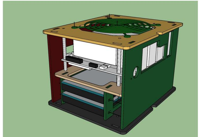
Figure 19 - Design prototype for ODRROID-H2 case
