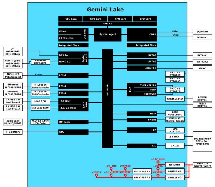
Figure 2 - ODR0ID-H2 Block diagram and interconnections.
