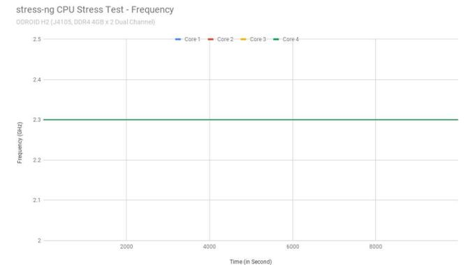
Figure 6 - ODROID-H2 CPU stress test results
