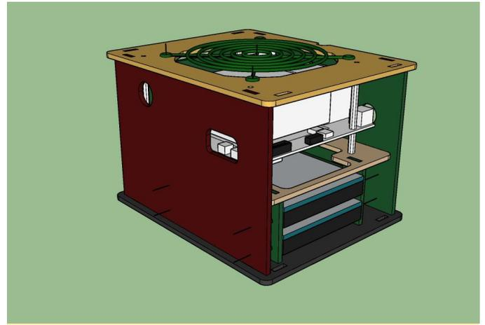
Figure 18 - Design prototype for ODRROID-H2 case
