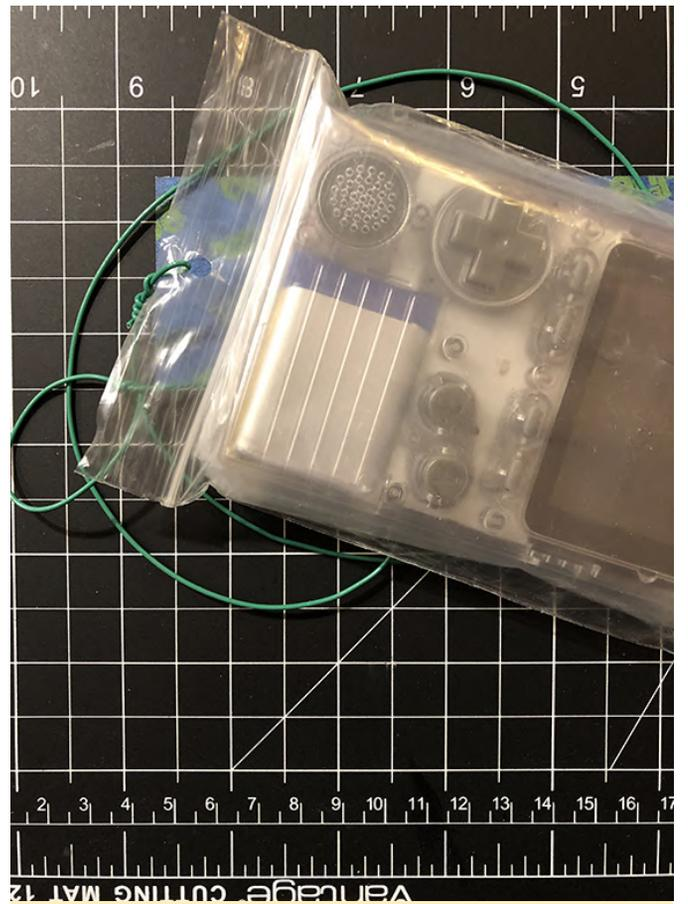
**Figure 5 - All ready to go outside and record data inside three zipper-lock plastic bags**
