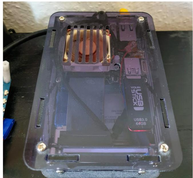
Figure 3 - XU4 cloudshell with Noctua cooler
