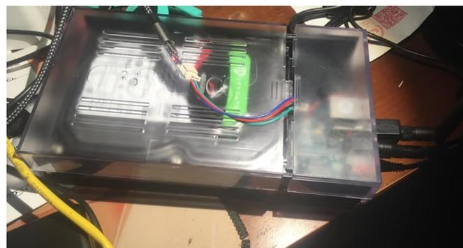
**Figure 3 - ODROID-HC2 being worked on at my desk with the UART connector kit pictured**
