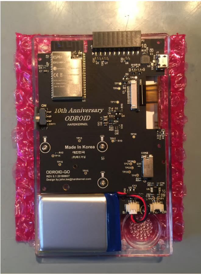
**Figure 8 - Example battery placement**
