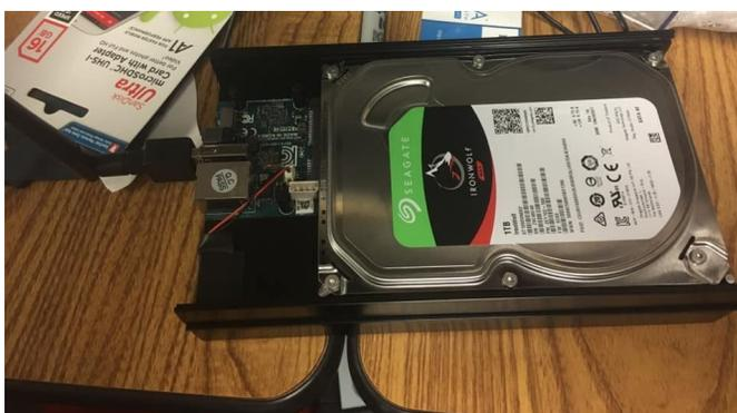
**Figure 1 - ODROID-HC2 with RTC battery, 1TB Seagate Iron Wolf HDD, and Model 3 Wifi NIC**
