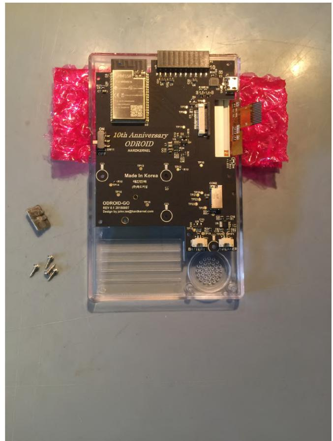
**Figure 5 - Placing the circuit board**
