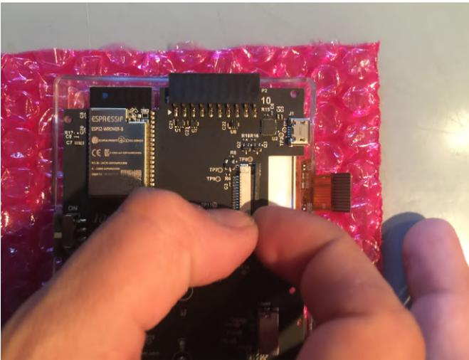
**Figure 6 - Hold the ribbon in place**
