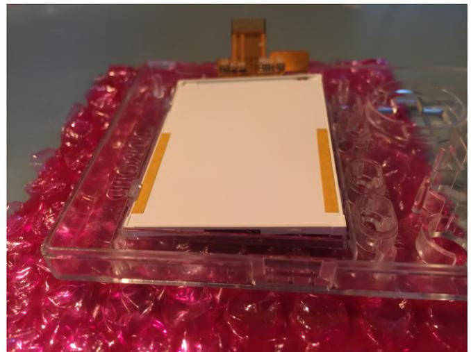
**Figure 3 - Snap the screen into place**
