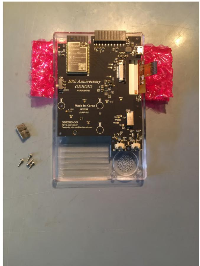
**Figure 5 - Placing the circuit board**
