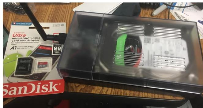
**Figure 2 - ODROID-HC2 pictured in a clear acrylic case with the wireless NIC inserted, and 16GB flash card before it was flashed with the Ubuntu 18.04.1 OS**
