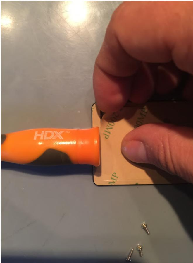
**Figure 12 - Peel out the adhesive strip**
