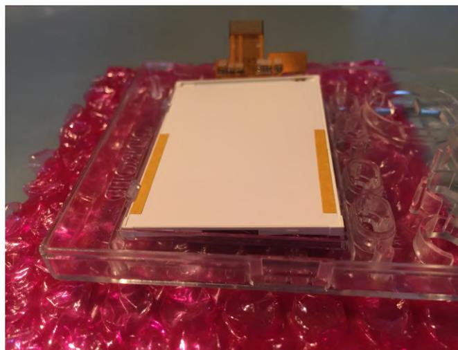
**Figure 3 - Snap the screen into place**
