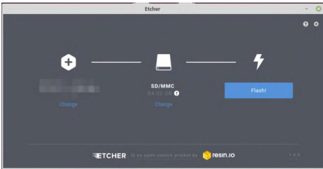
**Figure 8 - Screenshot of setting up Etcher to flash the SD with the OS**
