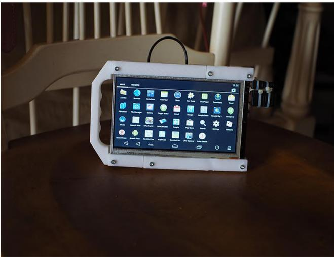
**Figure 2 - Switching jumper J1 converts the ODROID tablet into a handheld Android 4.4.4 device.**
