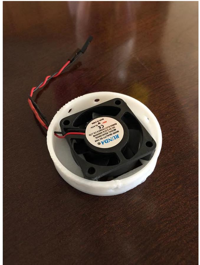
**Figure 5 - The optional USB fan can now be connected to the GPIO 5V power pins.**
