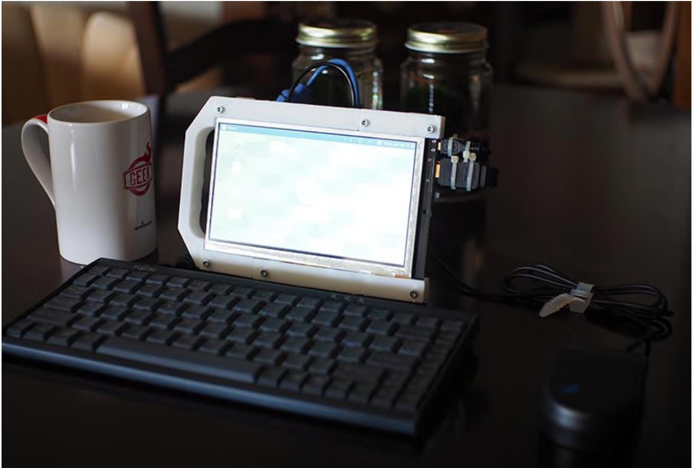
Hiding in plain sight in the powerful Hardkernel single board computer (SBC), the unassuming ODROID-C0. Slightly larger than a 3,000 mAh battery pack yet powered by a power-sipping Amlogic S805 System-on-a-Chip (SoC) featuring 1Gb of RAM, dual USB (2.0) ports, an eMMC interface, and a microSD storage card socket, this SBC is the best-kept secret in the ODROID world.
