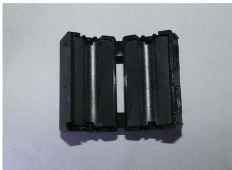
^ Clamshell-style ferrite chokes can be clipped to the ends of cables to reduce radio frequency interference.
