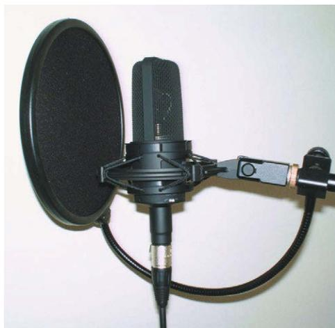
^ Basic pop filters still comprise nylon stocking fabric stretched over a metal loop, positioned in front of the mic.
