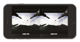
With a mobile phone you can create a stereoscopic display for use with a simple Cardboard viewer.
