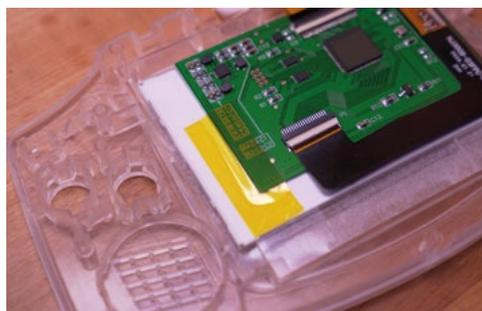
^ **Figure 14:** Taping the driver board to the back of the IPS panel keeps it from shifting around and makes the installation easier.
