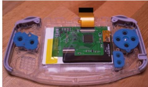
^ **Figure 17:** Everything in place prior to installing the motherboard.
