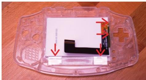
^ **Figure 10:** Be sure to orient the IPS panel as shown.
