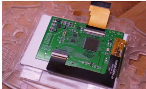
^ **Figure 13:** IPS panel connected to the driver board.
