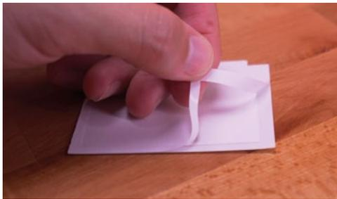
^ **Figure 7:** Peel away the release liner to expose the foam gasket adhesive.
