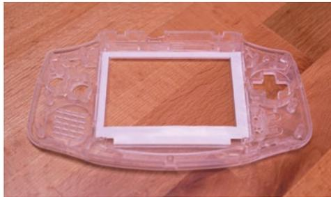
^ **Figure 8:** Be sure the gasket is oriented correctly within the LCD cubby. The thinner border is on the left and the thicker border is on the right.
