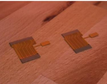
^ **Figure 11:** 40-pin ribbon cable is on the left and the 32-pin is on the right.
