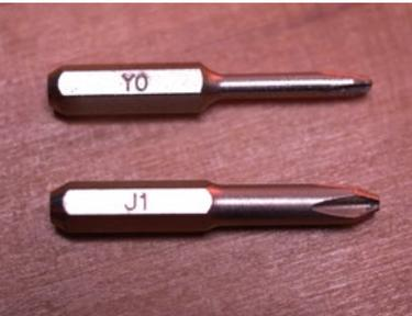
▲ **Figure 3:** The Y0 bit is primarily used on the exterior of most Nintendo consoles to deter consumers from getting inside. Internal screws are typically Japanese International Standard (JIS) – see box on page 55 for more info.
