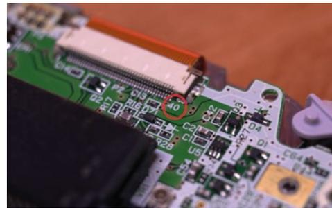
▲ **Figure 5:** Marking to indicate whether you have a 32 or 40 pin motherboard. This will dictate which ribbon cable you'll need for the backlight kit.
