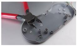
Figure 11: We can now start to trim away the unwanted pieces of plastic from the two halves of the case.
