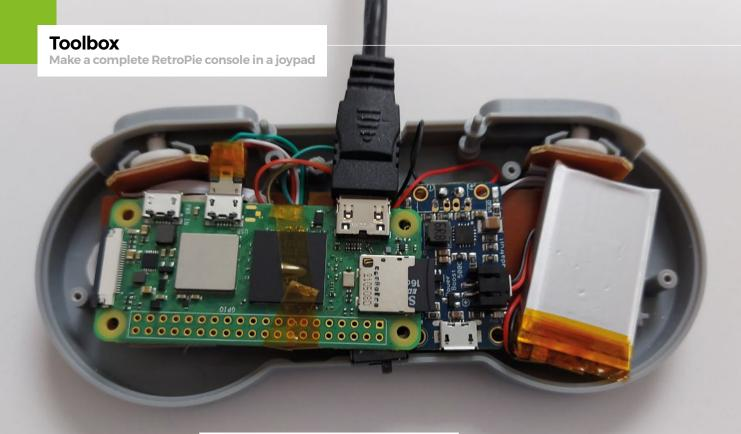
Figure 10: Here's how all the parts need to fit inside the controller.
