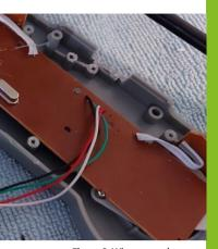
Figure 2: When removing the existing USB cable, be sure to leave about 5 cm of the coloured wires behind.
