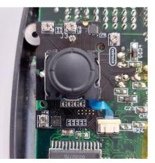
The RetroSticks GG soldered in place. Those screws around the edge of the device are used for calibration.
