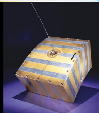
UPSat was built from the ground up, rather than relying on off-the-shelf subsystems – it was designed, as far as possible, to be reproducible by other teams using the types of tools and electronic equipment found in most hackspaces. With seven solar panels charging three cells, UPSat also had an on-board imaging system, a science unit with apparatus for measuring plasma, and its physical chassis was an interesting hybrid of aluminium and carbon-fibre-reinforced polymer panels.
