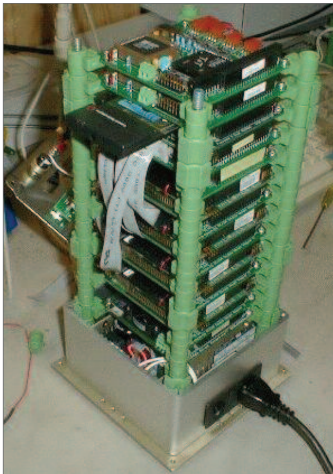
Figure 1. Minicluster I used four Pentium-based single-board computers (courtesy Sandia National Labs).
