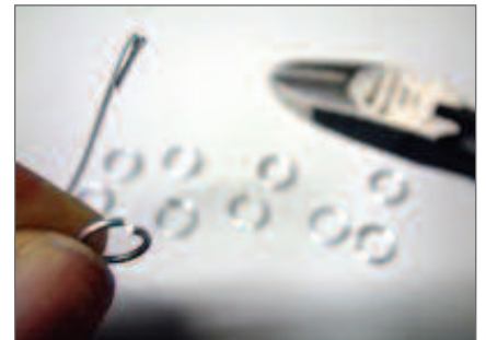
Figures 9–11. Medieval solution to a 21st-century hardware problem: wire spacing rings constructed chainmail-style (courtesy Josiah England).
