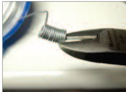
Figures 9–11. Medieval solution to a 21st-century hardware problem: wire spacing rings constructed chainmail-style (courtesy Josiah England).
