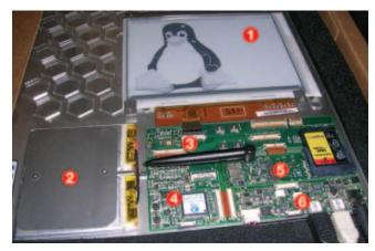
Figure 3. Picture and Block Diagram of the Hardware: 1 E-Ink Vizplex Display, 2 Li Ion Battery, 3 Display Adapter Board, 4 Metronome Display Controller Board, 6 Gumstix Board and 6 Lyre Mainboard
