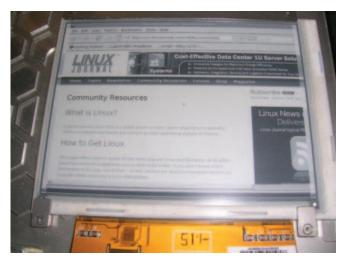
Figure 1. Firefox Displaying Linux Journal on an E-Ink Display
