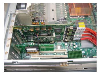
Figure 4. 3ware RAID Controller with Remote Battery Option
