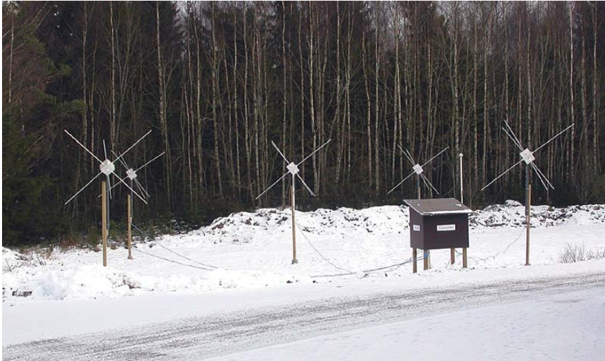
Figure 2. One of the test stations that gathers data for the Uppsala University Project. This station is located in Växjö, Sweden. It includes tri-pole antennas and three-channel digital sensors along with a GPS antenna and receiver.
