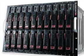
Blade server with, Highest computing density (20 DP nodes and 2.56TB mempy in 7U) Fastest and Most Cost-Effective Networking Solution (Infiniband DDR/QDR support)
