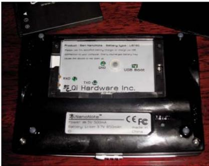
Figure 3. The Ben NanoNote's battery compartment—the round thing in between the GND and USB Boot pins is the nub used for shorting the two USB Boot pins together.
