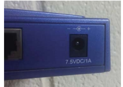
Figure 1. This network switch shows a need for 7.5V of DC current.
