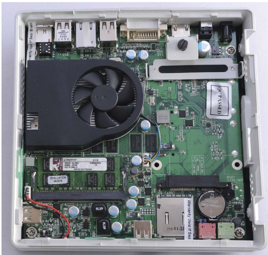
Figure 4. HD-ID11 motherboard with 2GB of Kingston RAM installed. Mount and thumbscrew is for the 2.5" HDD/SSD.
