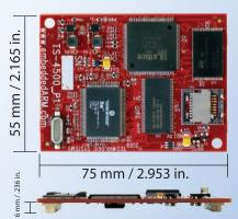
TS-SOCKET Macrocontrollers are CPU core modules that securely connect to a baseboard using the TS-SOCKET dual connector standard with common pin-out interface. COTS baseboards are available or design your own baseboard for a custom solution with drastically reduced design time and complexity. Start your embedded system around a TS-SOCKET Macrocontroller to reduce your overall project risk and accelerate time to market.
