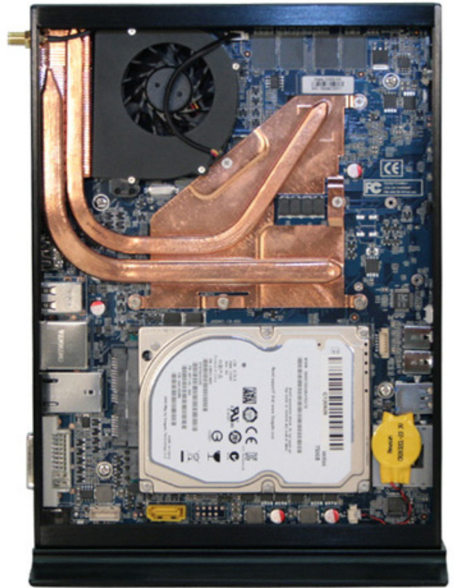
Figure 3. The compact design necessitates the well-placed heatsink (photo from http://polywell.com ).
