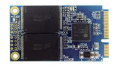
16GB to 128GB, the mSATA SJ2 SSD with SATA-III interface offers extremely fast speeds of up to 480MB/sec reads and 160MB/sec writes for mobile solutions. A small form factor and high reliability are other features that Super Talent notes about the mSATA SJ2. Target applications include aerospace, casino gaming, embedded systems and the medical industry.
