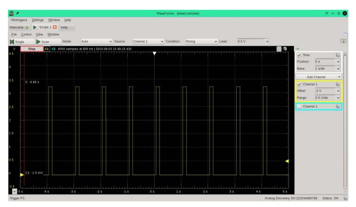
Figure 3. PWM Signal Output
