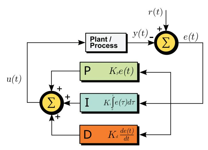
Figure 4. PID en updated feedback by TravTigerEE—Own work. Licensed under CC BY-SA 3.0 via Commons.
