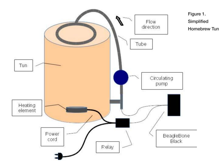
of 1800 W (Figure 1). Helped by a circulating pump, the mash (fluid) circulates from the bottom of the tun to the top overflowing the malt.
