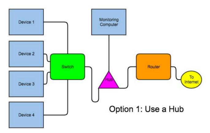
Figure 3. A hub is technically an option, but not a good one.
