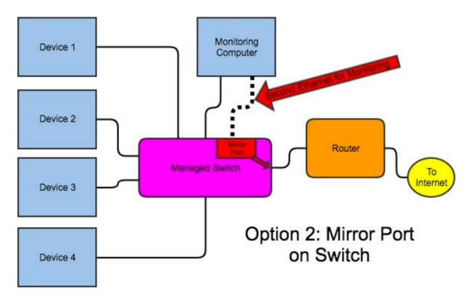
Figure 4. This is probably the best way to monitor traffic, but it requires a managed switch, which I didn't have.
