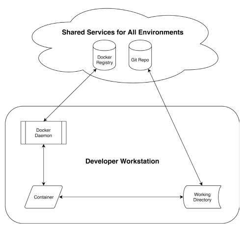
Figure 2. Idealized Docker-Based DevOps Pipeline
