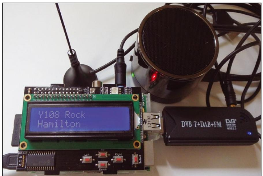
**Figure 4:** LCD FM radio control.
