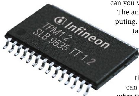
Trusted Computing environment is a small hardware component called a Trusted Platform Module (TPM). The TPM is a chip connected by bus to the system motherboard, and sometimes it can be retrofitted as a module (Figure 1). TPMs are not fast or powerful – almost anything that can be done on a TPM can be done much faster on the CPU. Neither can the TPM see what's happening on the rest of the system; TPMs know only what the rest of the computer chooses to tell them.
