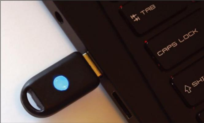
**Figure 1:** The first part of Signet is an external USB device, which must be present for a login to work.
