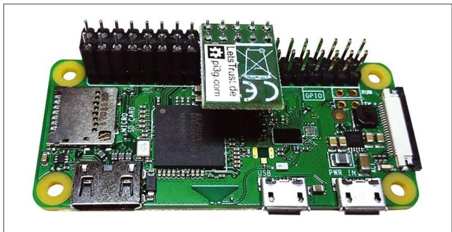
**Figure 1: LetsTrust provides an attachable TPM 2.0 module for the Raspberry Pi.**
