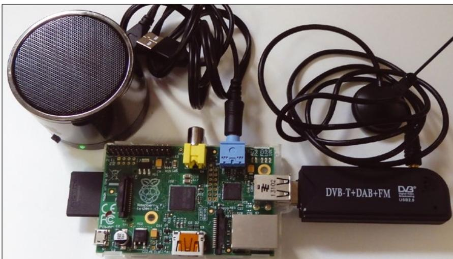
**Figure 1:** FM radio hardware setup.
