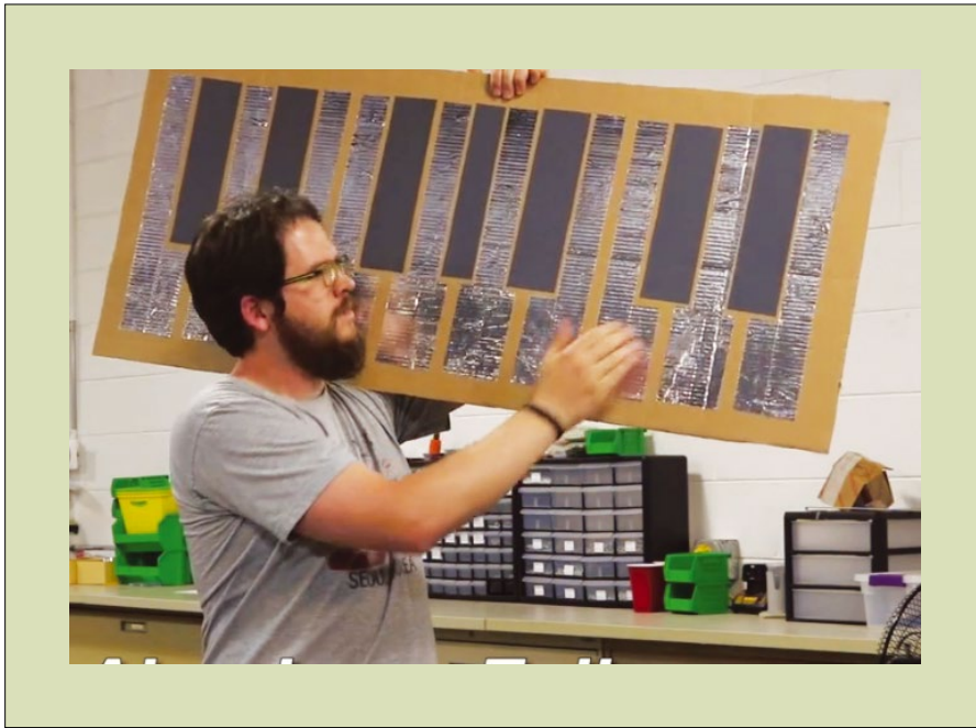
Figure 5: Using conductive tape to produce a playable keyboard.
