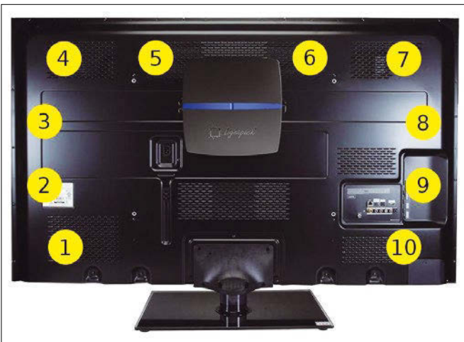
Figure 2: In the "Andromeda" arrangement, you attach the LED strips clockwise from the bottom left.
