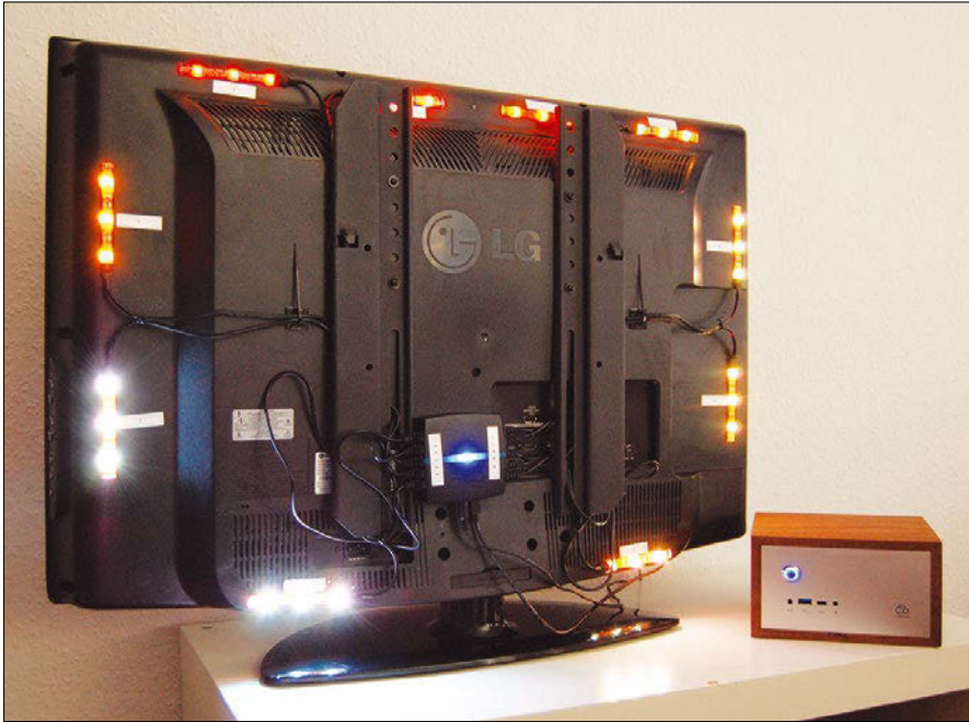
Figure 1: The complete Lightpack kit mounted behind a TV set. A classic PC delivers the image data.
