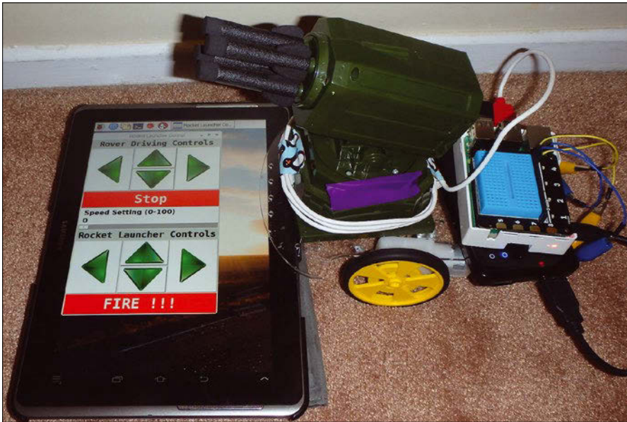
Figure 7: Tkinter-controlled rocket launcher.
