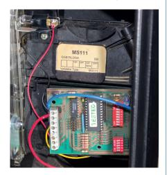
Our programmable coin mechanism is a Mars MS111. It accepts 10p, 20p, 50p and £1 coins and will send credit pulses at regular intervals to the JAMMA connector.
