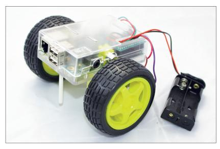
Though not strictly necessary, a portable USB power supply will let you run your creation untethered, and a Wi-Fi dongle will enable you to communicate with it once it's free.
