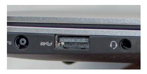
There are two charge friendly USB 3 ports, a combination mic/headphone jack and a mini-display port. An SD card slot would have been handy.
