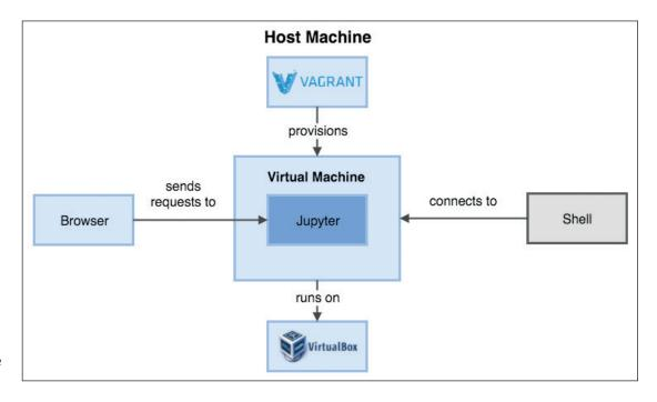
Both Vagrant and VirtualBox run on your host, with the Browser and a shell accessing the virtual machine using http and ssh. Inside the VM, the Jupyter server runs the IPython notebook. Afterwards, you should be able to run
