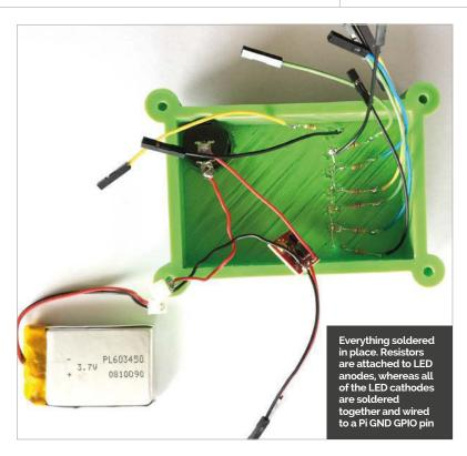
connection. Likewise, for the remaining LEDs, bend and solder each LED cathode to the next until you reach the 'Ready' LED. Stop at this LED. Do *not* solder the power (PWR) cathode to this chain: it must be connected to its own GND pin.
