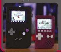
It's been through a few iterations, and the latest Pocket PiGRRL uses a Raspberry Pi and PiTFT HAT (320×240 pixels) to create a portable gaming console.
