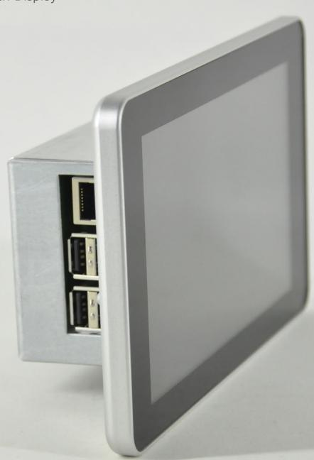
Raspberry Pi 3 Raspberry Pi Touch Display Strato Pi board Power Supply 12-28VDC Real Time Clock Buzzer Optional RS232/RS485 & UPS Aluminium and steel rear chassis Brushed aluminium front bezel Optional back box for wall mount
