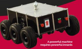
**JUDGES ((** The monster truck of SAY robots: with a 12V battery, six wheels, and three horsepower, it's strong enough to carry a person!"
