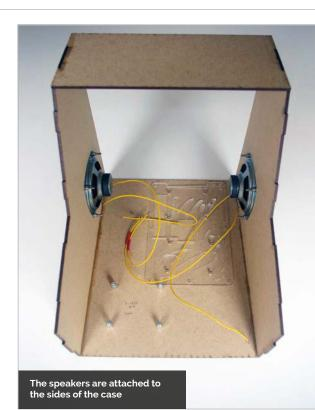
it meant we could mount the LCD driver board and Pi very easily, but it's equally easy to add your own mounting holes and standoffs. In our build, we used a small drill bit to add several mounting points on the base unit, so that we could install standoffs for the Picade PCB, as well as holes for the two speakers.
