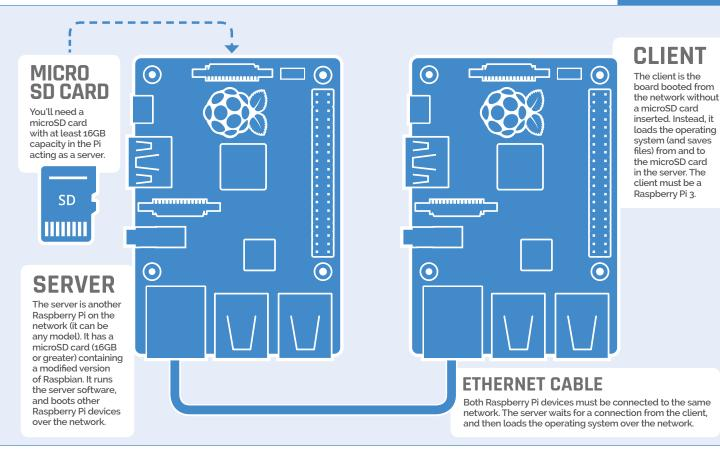
Place the microSD card into the client Raspberry Pi (the Raspberry Pi 3 that you intend to boot over the network and without the card in future).
