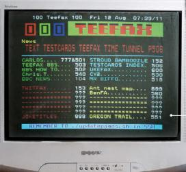
The data transmitted via the Pi's composite video signal is converted into teletext pages
