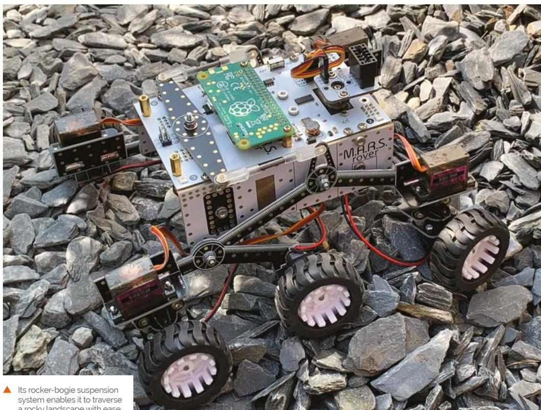
▲ Its rocker-bogie suspension system enables it to traverse a rocky landscape with ease
