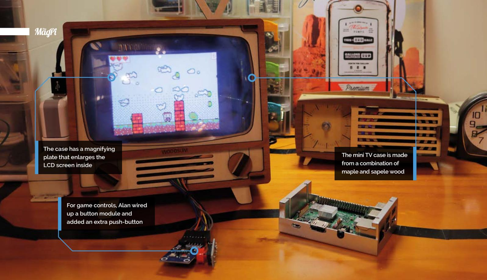
The case has a magnifying plate that enlarges the LCD screen inside
