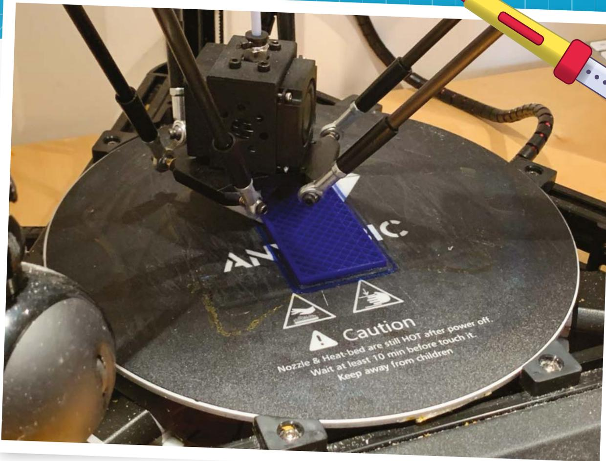
a big fan of OctoPrint here, especially running on a Raspberry Pi). We printed our parts in PLA on an Anycubic Kossel Linear Pro at 0.2 mm resolution, which is a nice balance between quality and speed. Remember to check your levelling first and give the print time to ‘settle’ once complete. Finally, never leave a 3D printer unattended.
