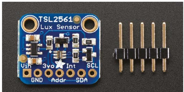
▲ The TSL2561 measures luminosity – the amount of light present – and also uses the I<sup>2</sup>C pins, so can share wires and pins with the BME280 sensor
