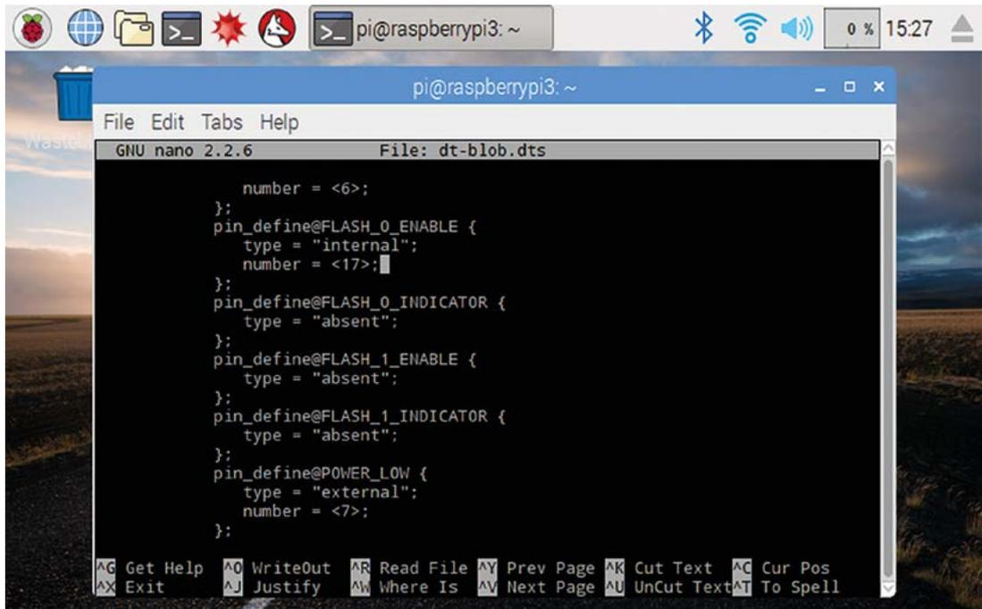
► You need to edit the device tree source to enable a GPIO pin for the flash
