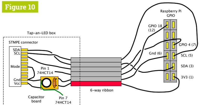
▲ **Figure 10** Wiring the 6-way ribbon cable to Raspberry Pi's GPIO connector
