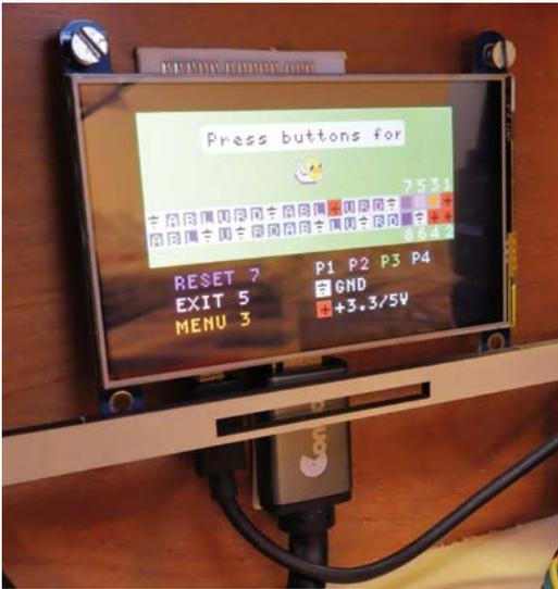
▲ A 4-inch LCD is connected via HDMI, but enlarged by the magnifying plate
