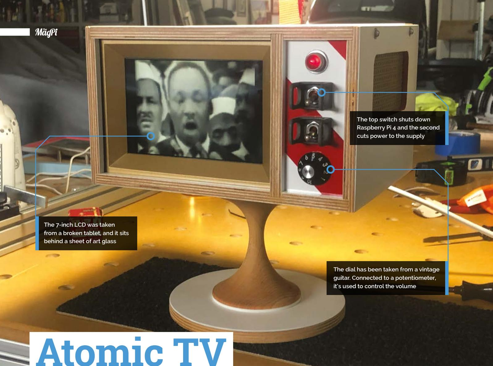
The 7-inch LCD was taken from a broken tablet, and it sits behind a sheet of art glass
