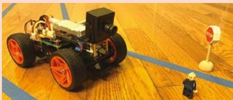
▲ David Tian has turned an off-the-shelf Pi-Car V robot into self-driving car using a Coral USB Accelerator ([magpi.cc/deeppicar](http://magpi.cc/deeppicar))
