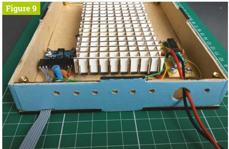
▲ **Figure 9** Fitting the two boards either side of the light baffles
