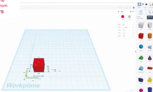
▲ Use the ruler tool to enable precise sizing of objects in the workplane
