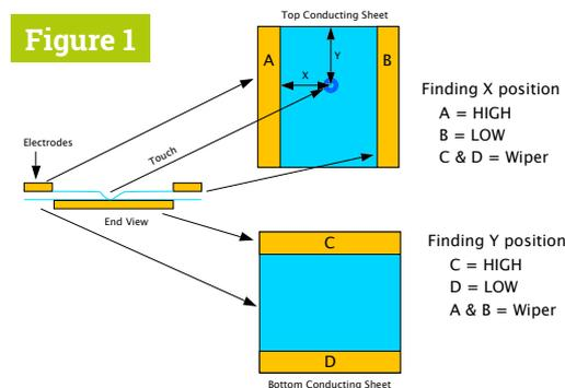
▲ Figure 1 How a resistive touchscreen works
