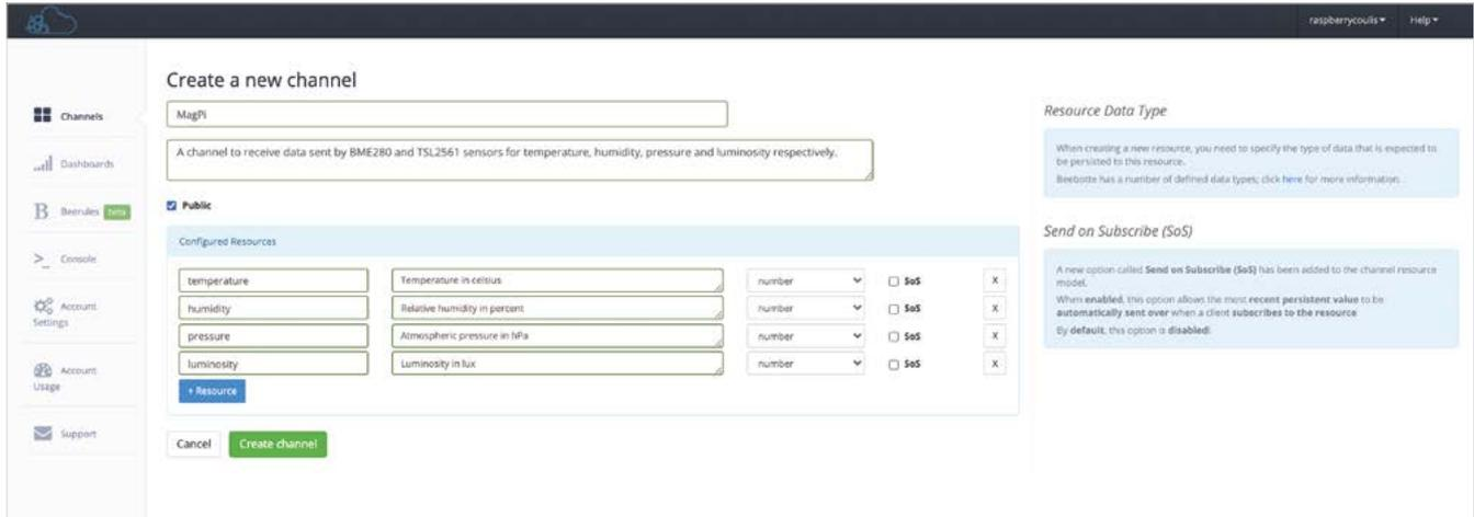
▲ A channel in Beebotte is required to receive the data measured by our sensors and sent by our Raspberry Pi so it can be visualised in a graph
