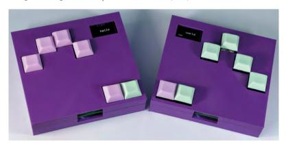
modeller to create the case. The positions of the keys and the case layouts are synchronised by Python code running inside KiCad and FreeCAD, allowing for flexible key positioning and ensuring that the holes for the keys match the key positions on the circuit board. You can find the designs, along with the C++ source for the keyboard, on the GitHub repository for this project here: **github.com/CrazyRobMiles/PICO-blue-chords**.
