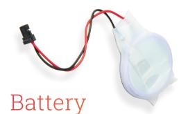
Raspberry Pi 5 has a two-pin JST (Japan Solderless Terminal) port marked BAT. This is used to connect a battery (or other power source) to the new Real Time Clock (RTC).
