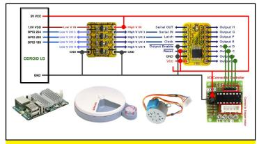
Figure 4 - ODROID Internet-controlled cat feeder schematics
