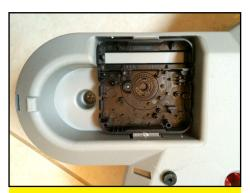
Figure 2a - Clock mechanism removed with lever gear visible
