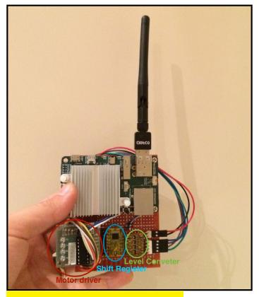
Figure 5a - Board with all components attached
