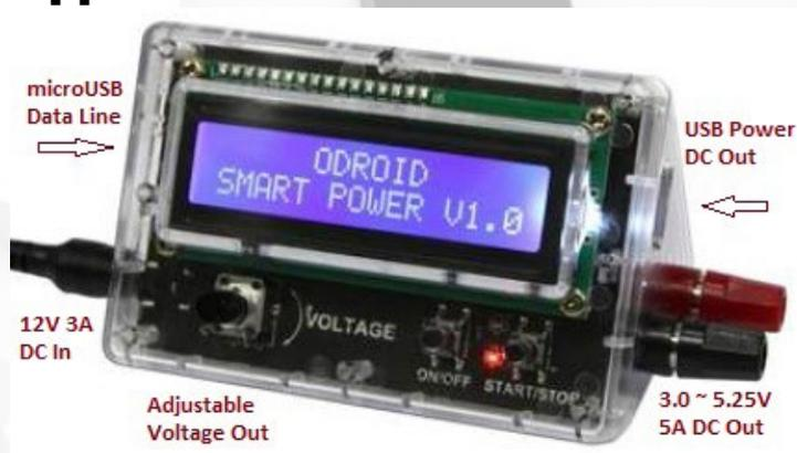
Hardkernel has developed an open source monitoring application called SmartPower that works with the Smart Power device. Although they have provided a pre-built executable binary, I'll describe the process of building the application from its source code. Follow the list of steps to create the build
