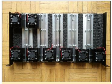
Preliminary design of the BOINC cluster, with the 40x40mm fans installed
