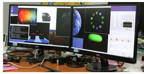
n this article, I'll demonstrate how to use two monitors to extend the desktop of an ODROID-XU3, as seen at ARM TechCon 2014. Each monitor can display the same image, or be configured to display separate images, allowing the 1920 x 1080 desktop to be extended to 3840 x 1080.
