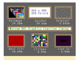
Graphical test on the ARM build of DOS-Box. This graphic tests gave odd results: some tests seemed to run faster with more colors and in higher resolutions, while others seemed normal
