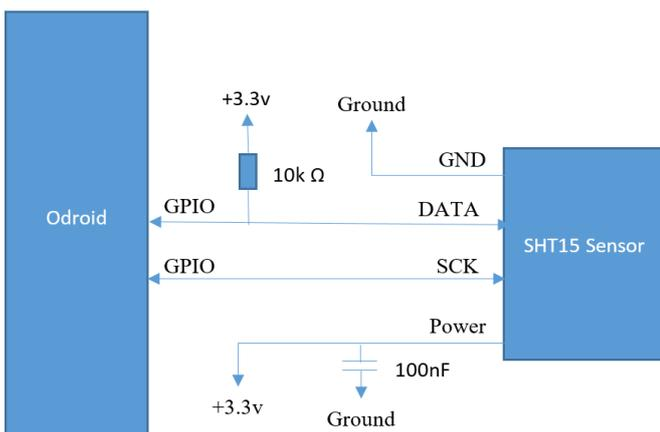
It's recommended by the manufacturer as a set-up that yields good measurements. Second, soldering an SHT15 is difficult. To make things easier, this tutorial uses a pre-manufactured SHT15 sensor board.
