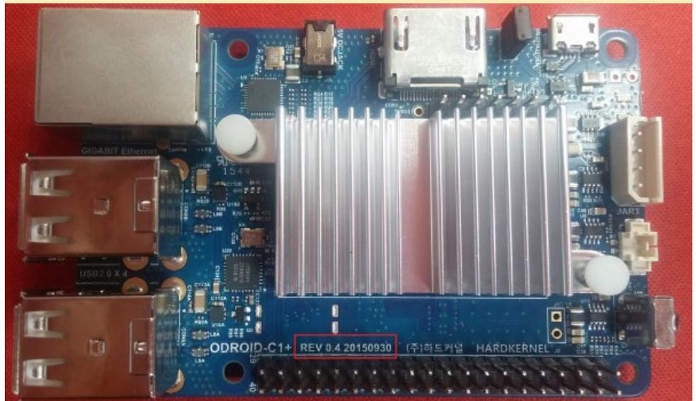
**Figure 2 - J8 jumper location on the latest revision of the ODROID-C1+**
