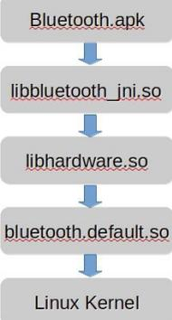
Programming Bluetooth is fun, but have you ever wondered how the internals work? How does the app that “communicates” with the lower level to enable my application send and receive data wirelessly? Figure 3 shows the high level view of what happens internally when you turn on Bluetooth in your device. Turning Bluetooth on manually is done via the Settings application in your Android device.
