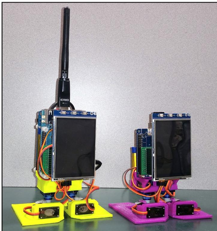
The OWEN assembled and in 2 configurations: wired and wireless,
