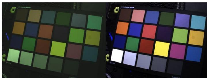
**Original color image obtained by using Bilinear Interpolation of Bayer image (left) and the color image enhanced through a proprietary enhancement algorithm (right) applied to the original image.**
