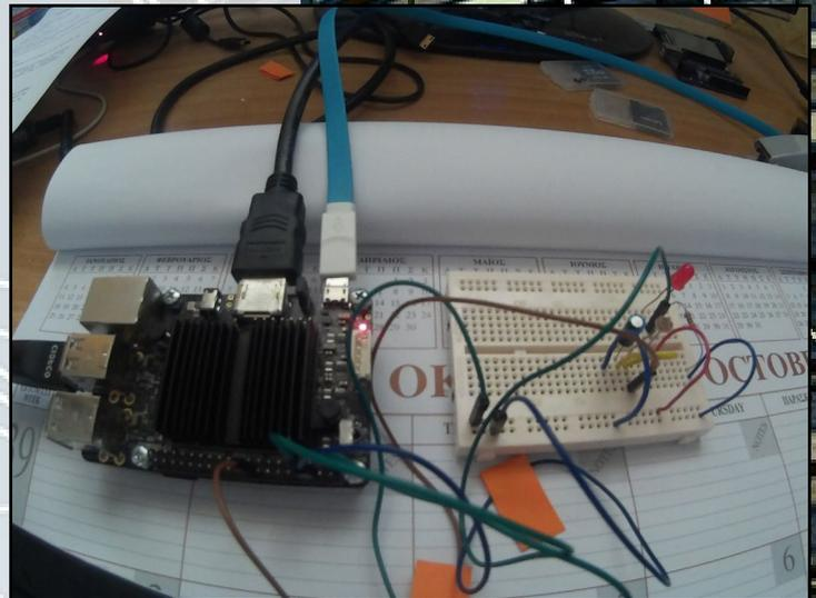
The assembled lighting solution using an ODROID-C2 and C Tinkering Kit
