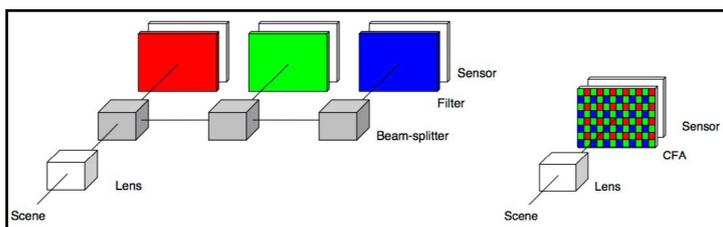
**Two different structures of color sensor: multi-color sensors(left) and single monochrome sensors(right)**
