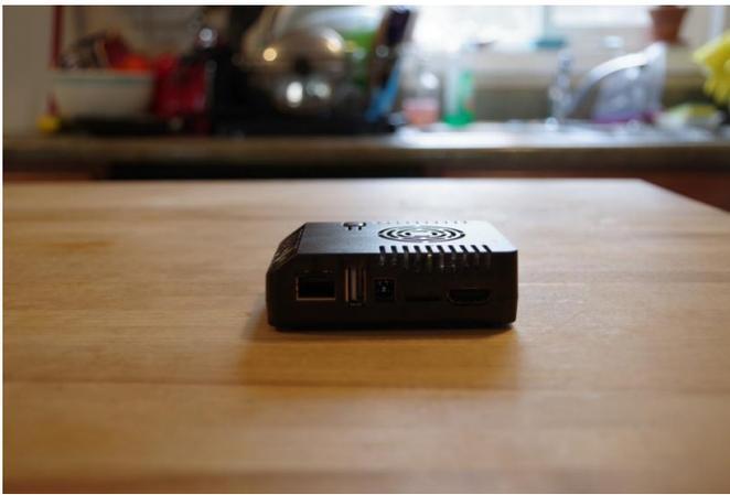
Installing Recalbox on the ODROID-XU4 is fairly simple. You only need the ODROID-XU4 board, a compatible 5V/4A power supply (PSU), eMMC module or microSD card running the ODROID-XU4 Recalbox image, and an optional but recommended case.
