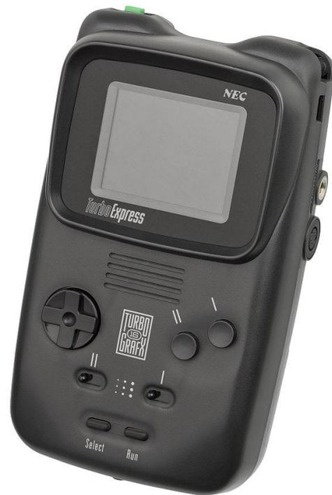
**Figure 7 - The PC-Engine GT / TurboExpress handheld version of the PC-Engine**
