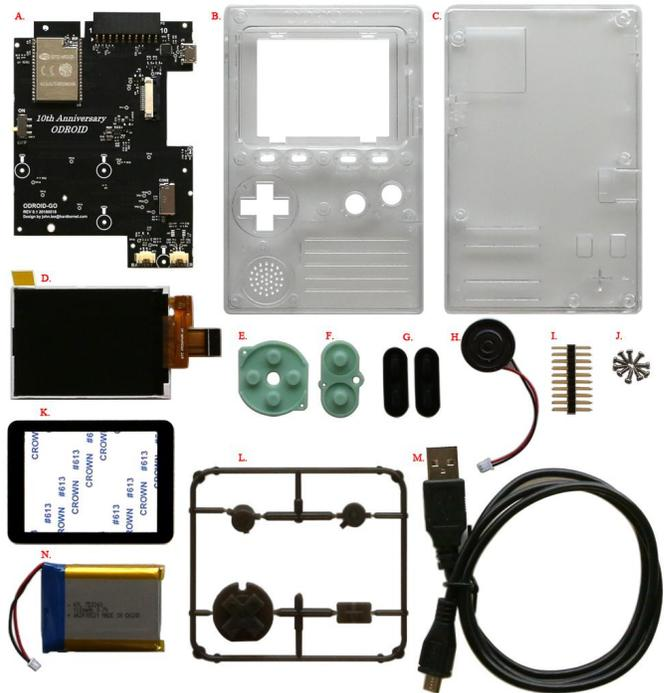
**Figure 6 - Parts included in the ODRROID-GO kit**
