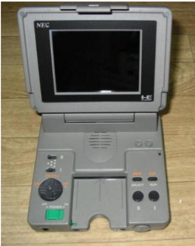
**Figure 6 - PC-Engine LT with built-in monitor and speaker**
