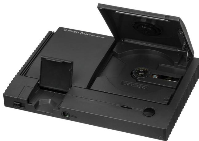
**Figure 4 - TurboDuo One console that already includes the CD-ROM add-on for the TurboGrafx-16**
