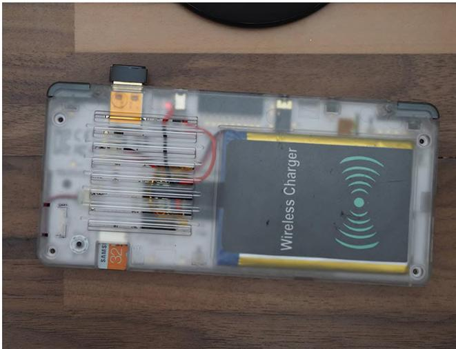
**Figure 2 - The wireless charger attached inside the ODROID-GO Advance case.**
