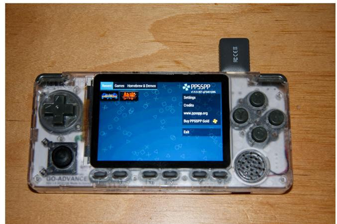
Figure 1 - ODROID-Go Advance running PPSSPP using SDL2 with screen rotation
