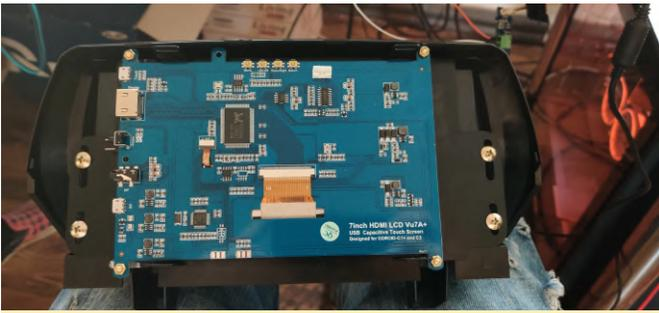
**Figure 2 - VU7a+ mounted inside dash casing**
