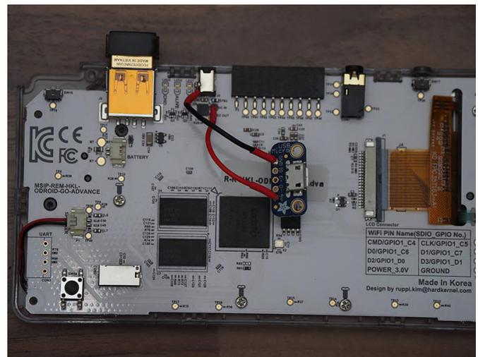
**Figure 1 - Closeup of the soldering required to add wireless charging to the ODROID-GO Advance.**
