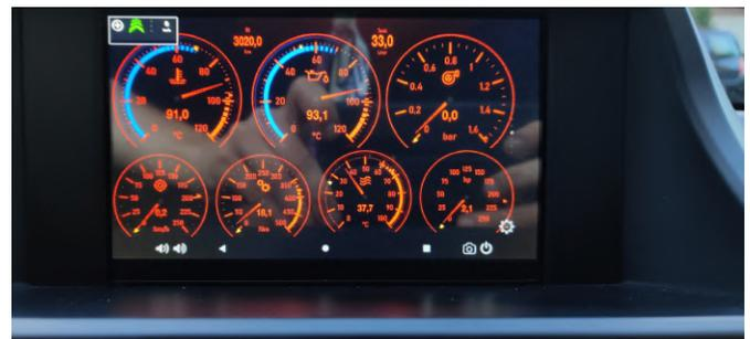
**Figure 1 - Fitted VU7a+ Display on the dashboard running Torque App**
